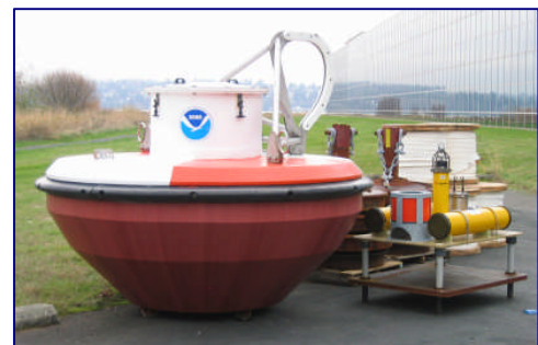
NOAA's DART II system includes a surface buoy (left) and bottom pressure recorder (right) to provide timely warning
