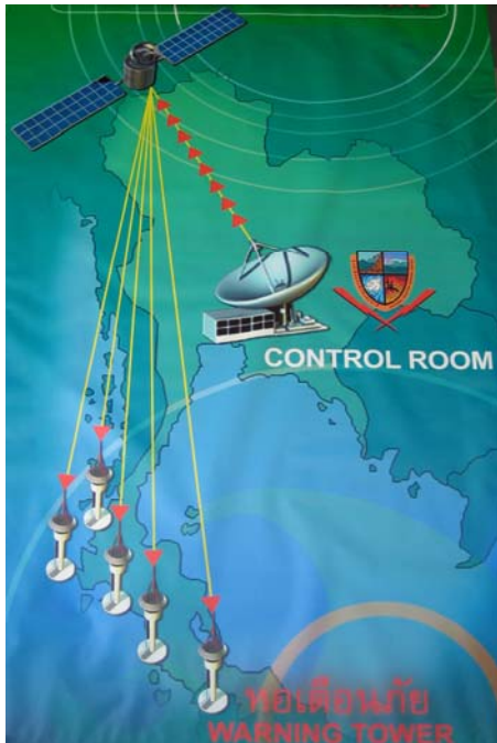
Figure 13: NDWC Diagram of Warning Tower Siren System for High Risk Coastal Regions. (Source: NDWC)
