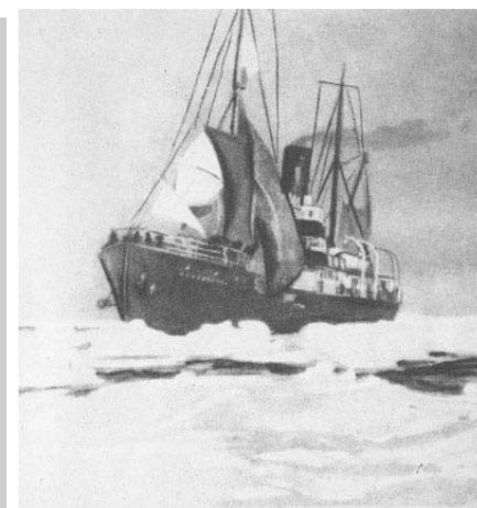
A. Sibiriyakov under jury-rigged sails after loss of propeller shaft near North Cape
