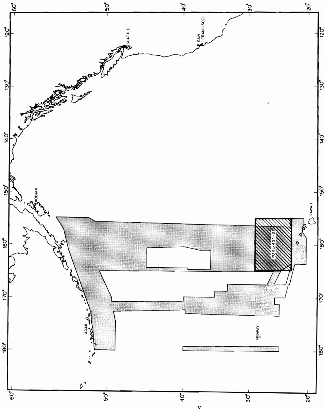
Figure 1. Location diagram for bathymetric map PORL-421-2. The extent of the SEAMAP survey completed with line spacing of 10 n mi as of January 1967 is indicated by shading.
