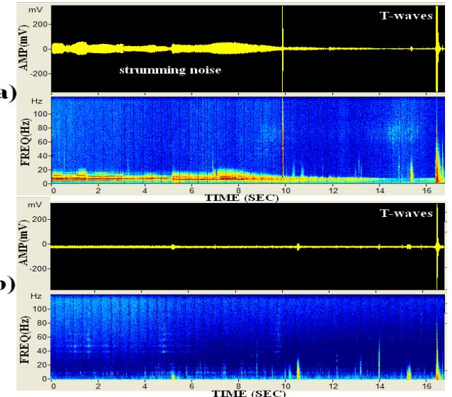
Figure 6. (a) Middle VAUH (@1000 m) record affected by the low-frequency strumming noise. The mooring line used was a 5/16" steel jacketed modem cable with smooth surface. (b) A regular VAUH record (M1) during the same time period is shown here for comparison. An elastic 5/16" Polyester line was used for mooring.
