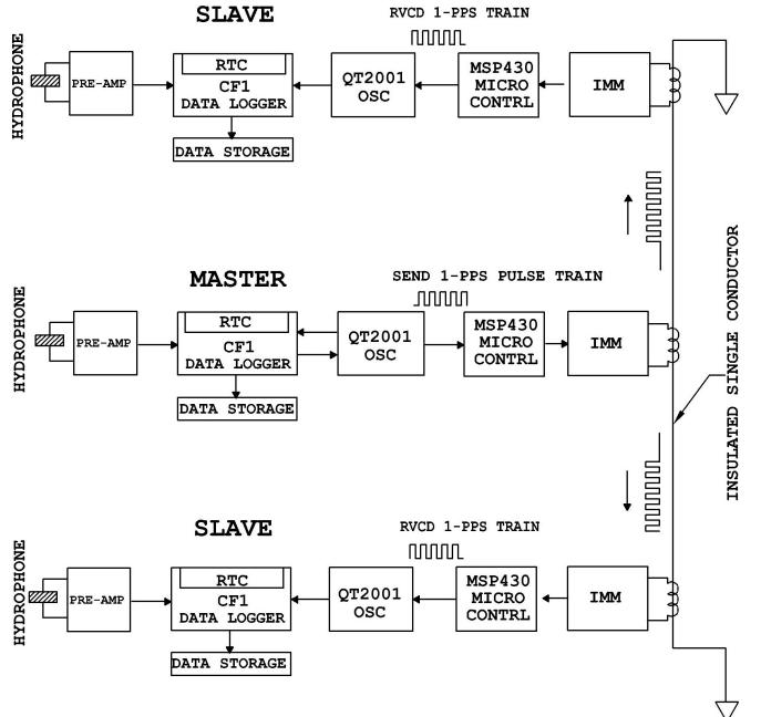
Figure 4. Block diagram of three VAUH units strung together for time synchronization.
