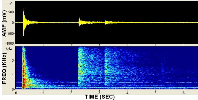
Figure 9. A 6.5-second long record of a typical glass sphere implosion recorded by the ship hydrophone on R/V *Kilo Moana* at 6-kHz sampling rate. A glass sphere of 14" diameter was imploded at 22°18'36"S-177°55'12"W at the depth of ~700 m. A direct arrival, bottom-bounded and surface multiples are seen in this picture.
