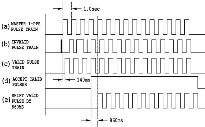
Figure 5. Master-to-slave VAUH timing synchronization scheme. Master's 1-PPS pulses are converted to *IMFlags* and sent to the slave units. Slave discriminates the noise, shapes the pulses and adds delay to compensate the transmission delay.
