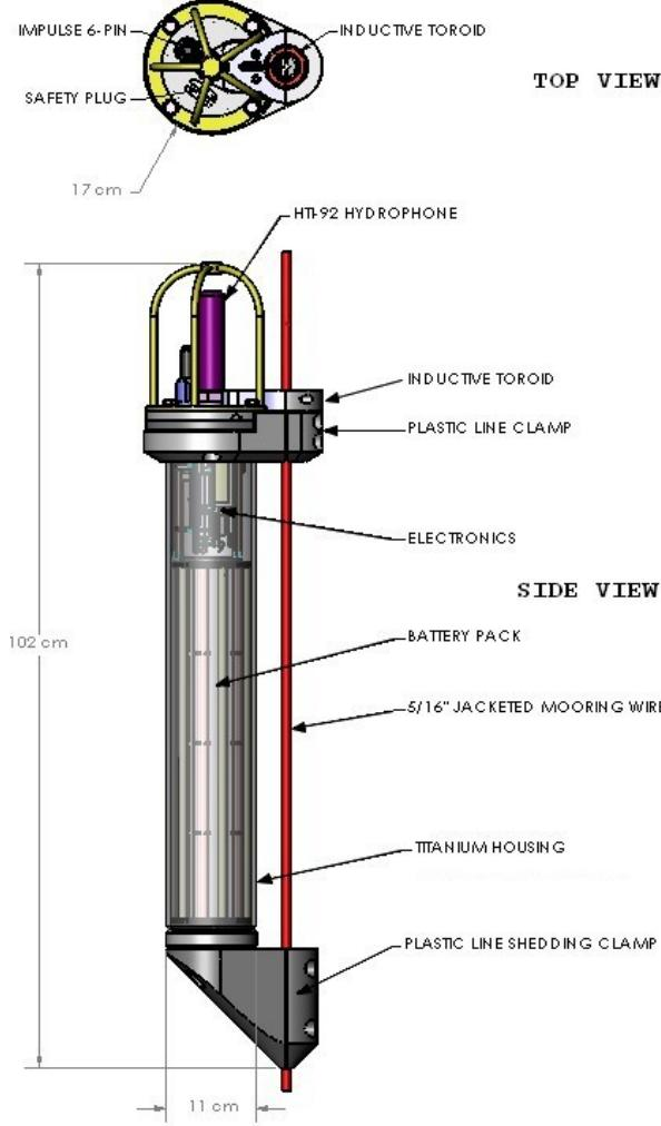
Figure 3. Assembly drawings of VAUH. A battery-operated electronics includes multi-processor data acquisition board with an inductive modem module, an 1.8" hard disk and an internal clock which is accurate to 1 sec/year. Multiple VAUHs can be strung together up to 1 km of separation from the master on the modem/mooring cable.
