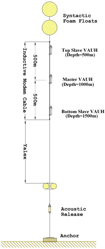
Figure 2. Mooring diagram of the vertical hydrophone array deployed in the Lau Basin.
