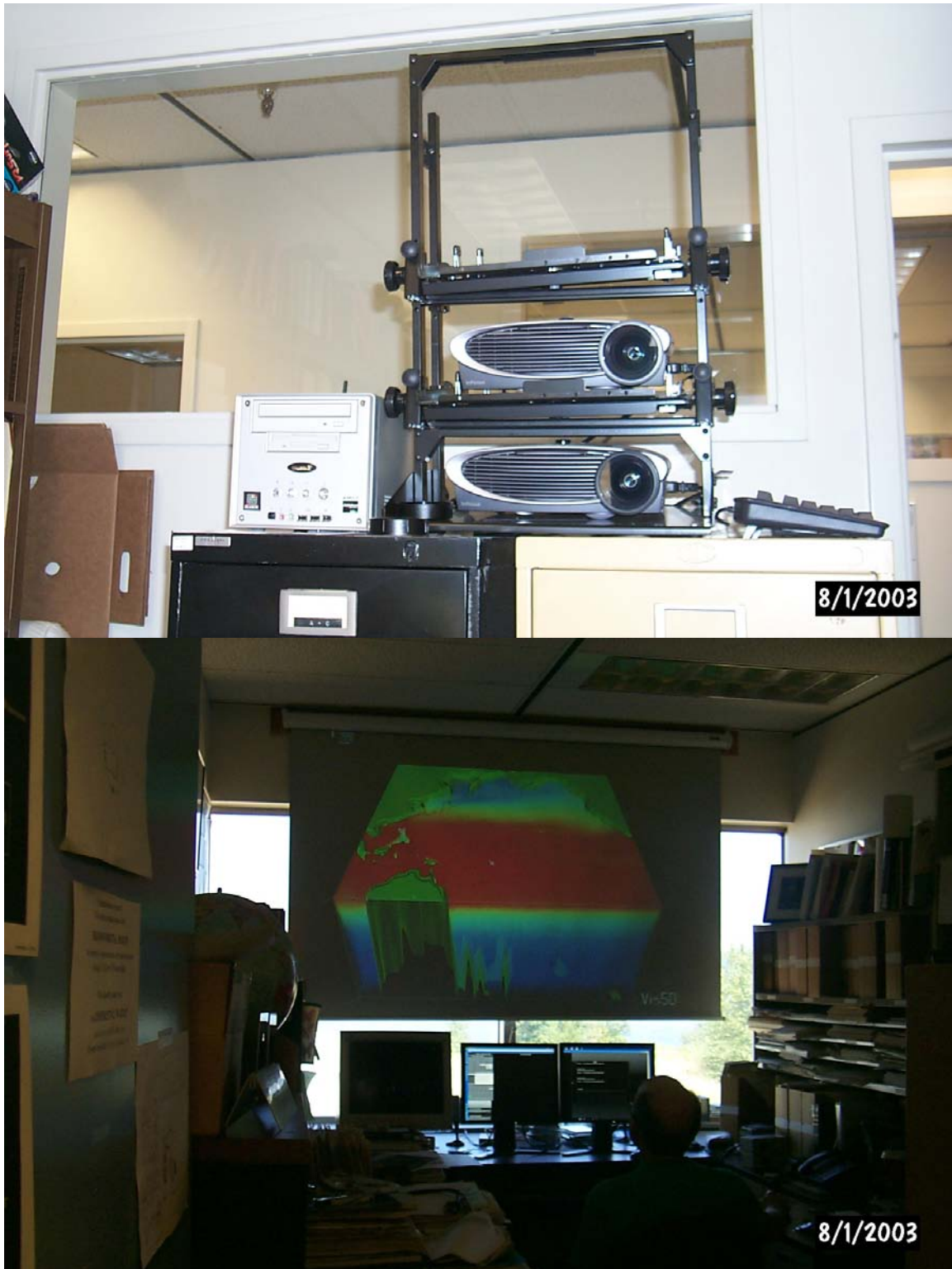
Figure 7. Setup of a Geowall system in a modest-sized office. Projectors with filters are placed at the back of the office, and driven with a linux PC outfitted with a graphics card supporting two displays. A polarization-preserving pull-down screen was installed in front of the window at the opposite end of the office. A model of the North Pacific (Curchitser et al. 2005) is displayed on the screen.
