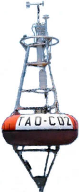
Version 1 is a TAO buoy, modified for the extreme conditions of Kuroshio Extension, with special sensors to monitor...
