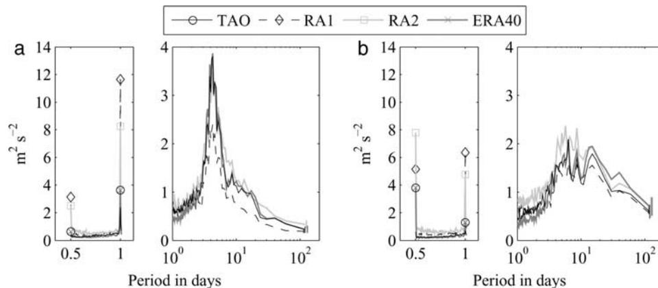
**Figure 1.** Power spectral energy of buoy and 1000 hPa reanalysis (a) meridional wind and (b) zonal wind for June–November 1992–2002 plotted in variance preserving format. Each figure is divided into two panels, one for the 12- to 24-hour time period and one for the 1- to 120-day time period. The 95% confidence limits for the lowest frequency (largest error) are shown as vertical bars staggered about 120 days for readability.
