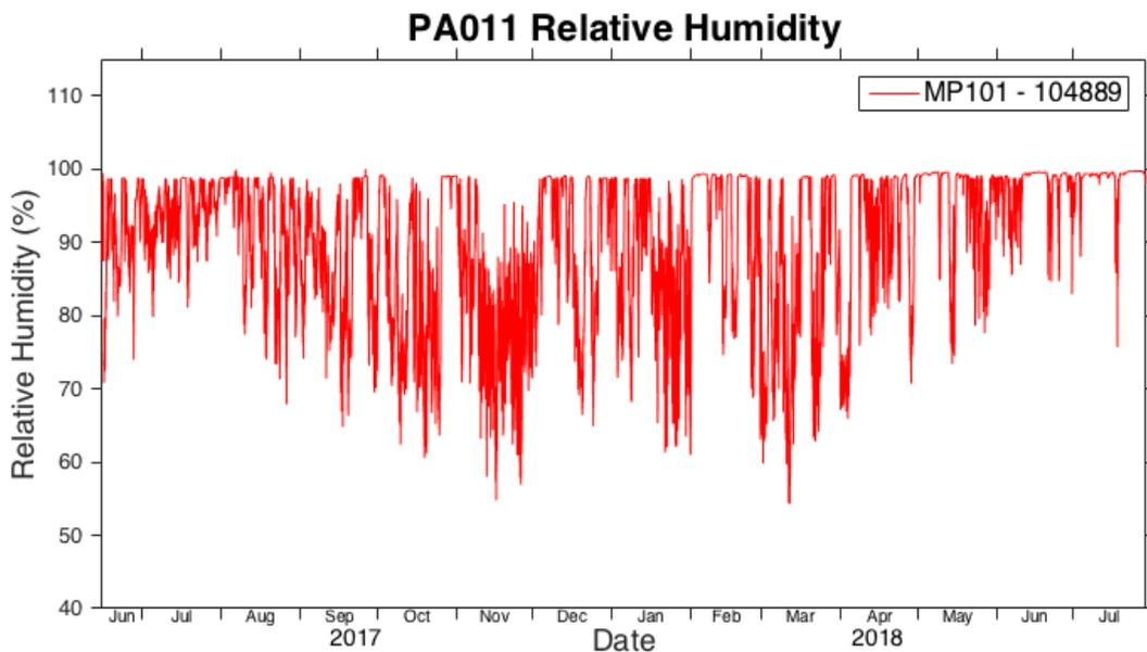
Figure C 5: Secondary (Flex MP101) relative humidity sensor. The instrument failed its post-calibration, so data were flagged as lower quality (Q4). The Hygroclip test sensor (not shown) failed its post-calibration as well, and both drifted with respect to the primary sensor.
