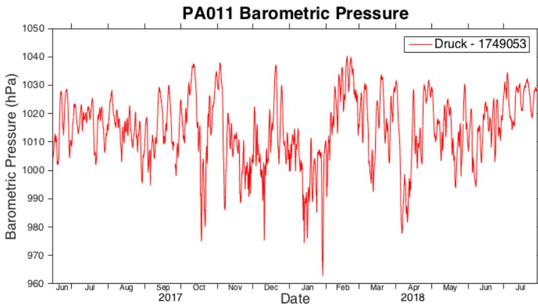
Figure C 7: Secondary (TFlex Druck) barometric pressure sensor. The data were biased high by about 0.4 mb compared to the Flex Paros. Field calibrations were unapplied, and new post-calibration coefficients were applied to the raw data to get this time-series. The adjustment aligned the data with the Paros to within accuracy specifications, and was flagged Q3 to indicate the adjustment.
