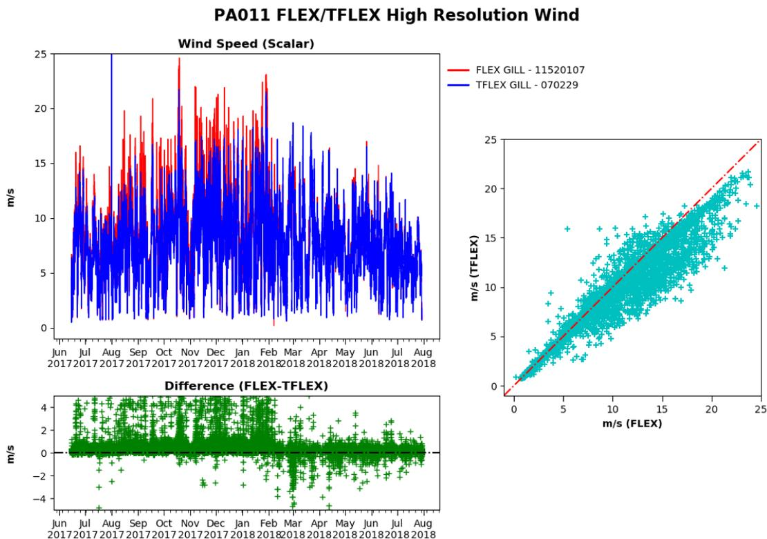
Figure 7: PA011 delayed-mode wind speed (before QC application), highlighting the Flex sensor bias.
