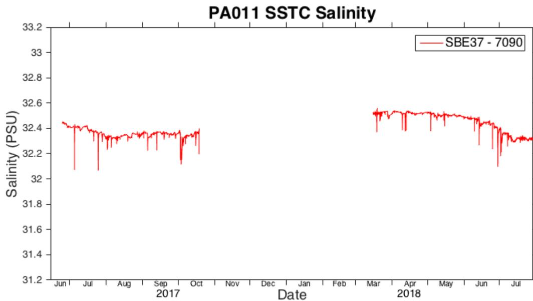
Figure C 9: Secondary (Flex) SSTC Salinity. Air bubbles likely infiltrated the SSTC, causing conductivity to drop close to 0 S/m mid-deployment. The erroneous conductivity, salinity, and density were flagged Q5 until the instrument recovered. If flagged data were shown here, values would quickly fall off the y-scale.
