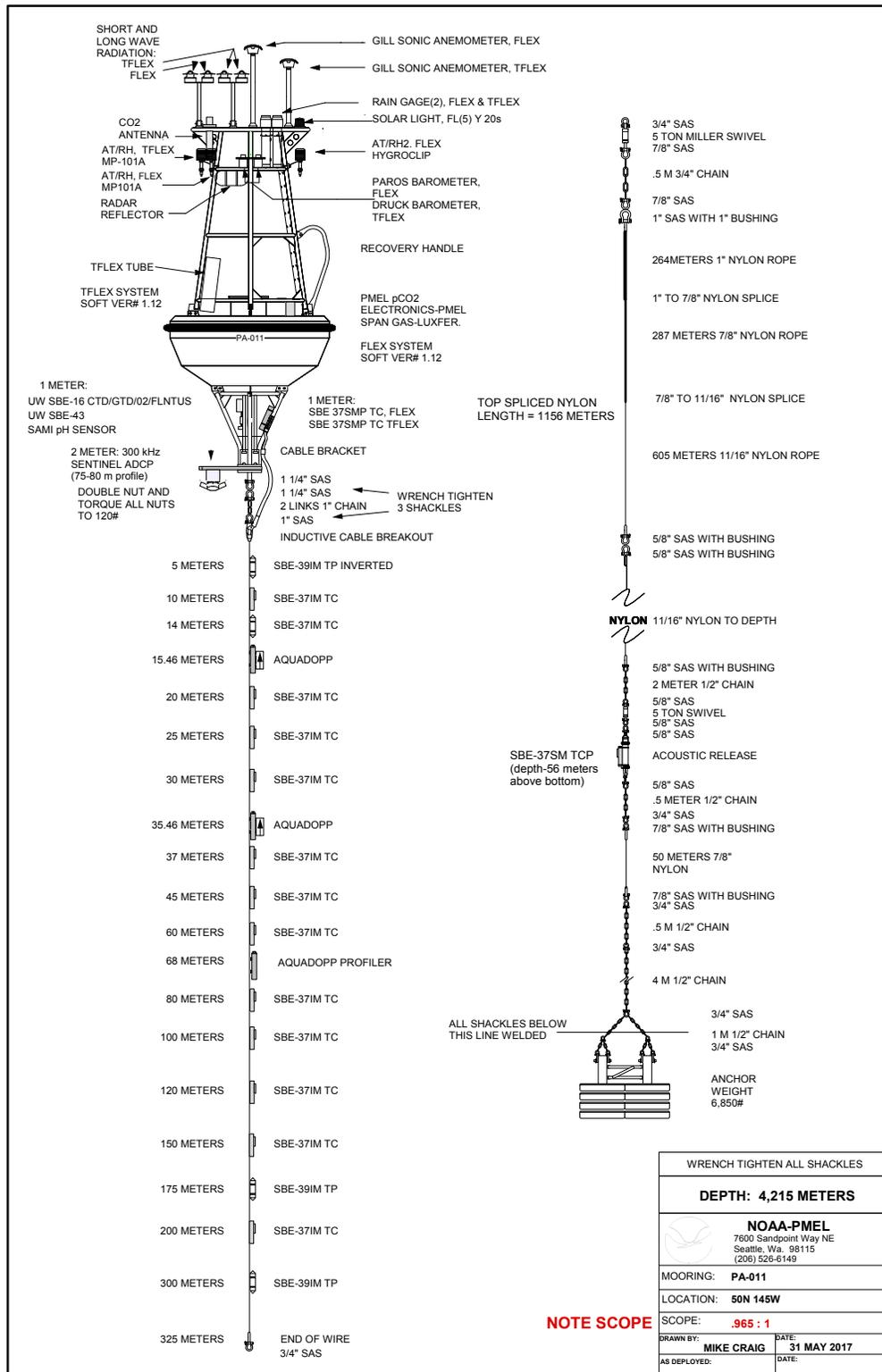
Figure 4: PA011 mooring diagram.
