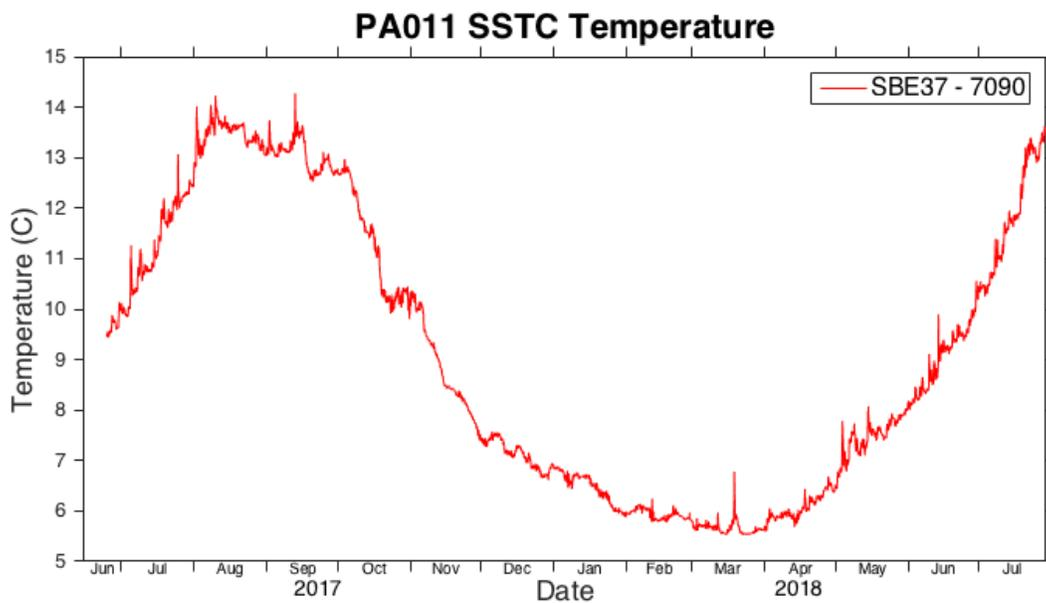
Figure C 8: Secondary (Flex) SSTC Temperature. This instrument turned on 10-days into the deployment, but data were otherwise unaffected.
