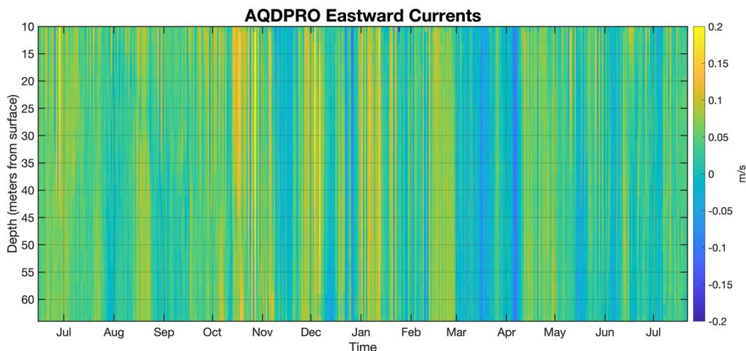
Figure 12: Aquadopp Profiler eastward velocities.
