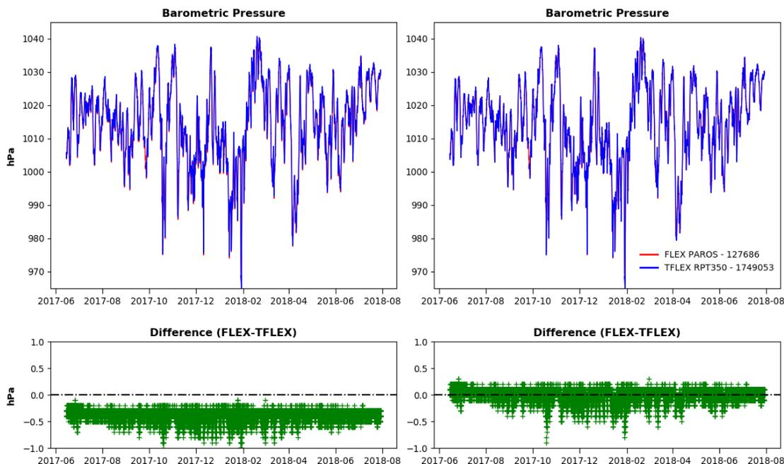
Figure 10: Flex and TFlex barometric pressure data. The application of pre-deployment calibration coefficients to the TFlex BP (left) resulted in a 0.4 mb offset, while the application of post-recovery calibration coefficients to the TFlex BP (right) brought the sensors within specifications.
