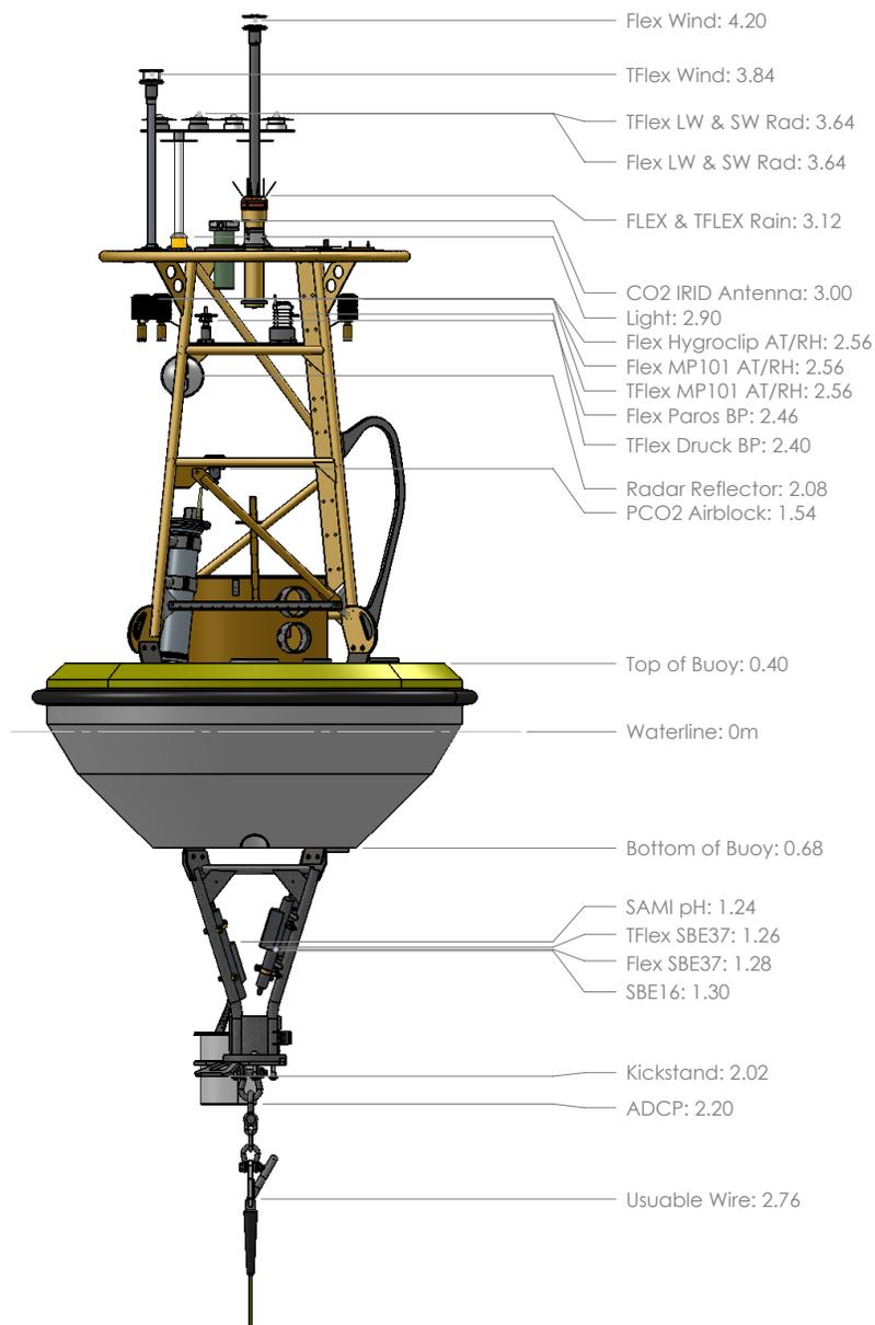
Figure 5: Buoy diagram showing bridle arrangement. The SBE16 package contains a suite of sensors.
