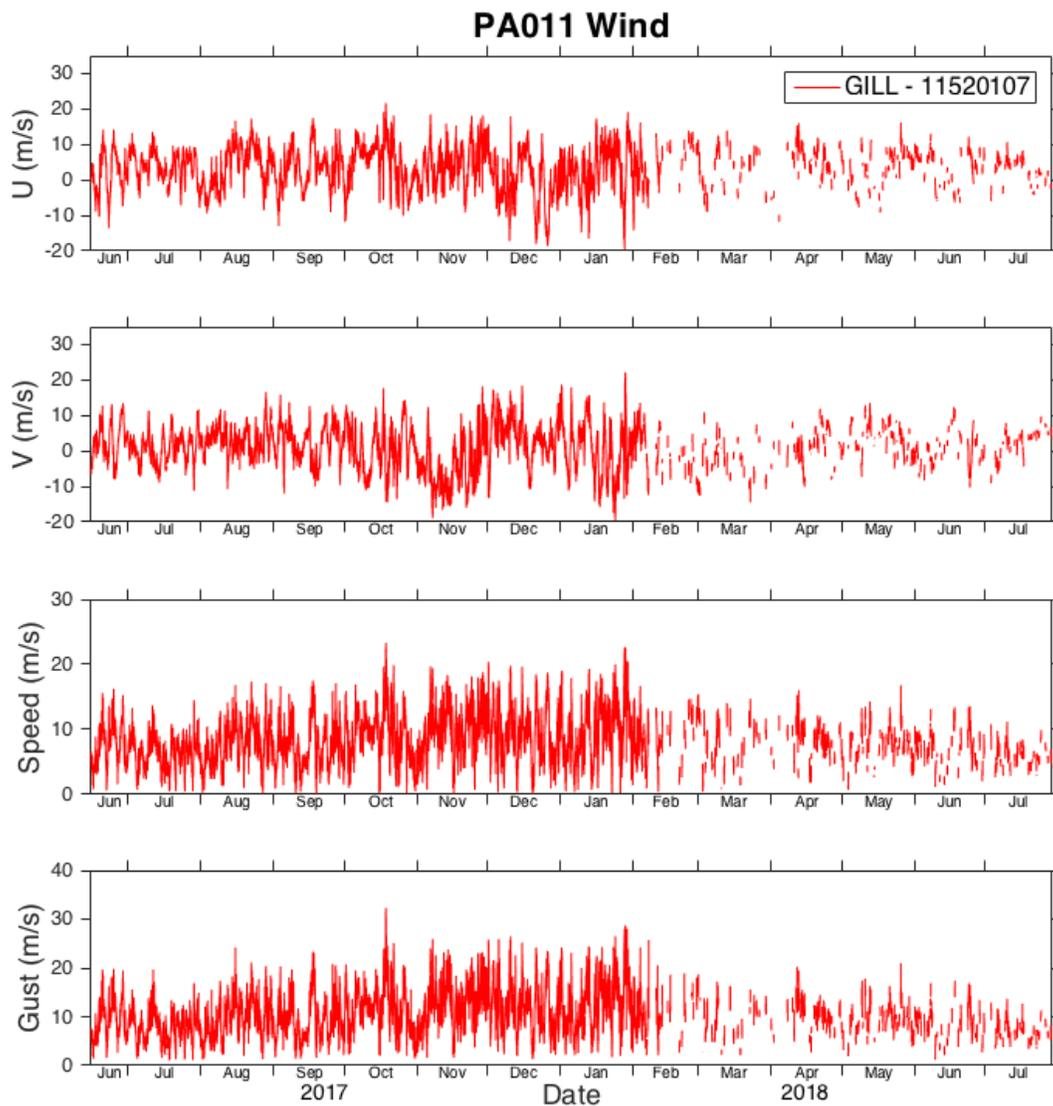
Figure C 4: Secondary (Flex Gill) wind sensor. Gaps in realtime and delayed-mode data occurred, especially in the latter half of the deployment, due to a combination of a failed compass post-calibration, large differences from the primary sensor (triggering gross error thresholds), and intermittency in the 240<sup>th</sup> sample. Data are flagged Q4 where present.
