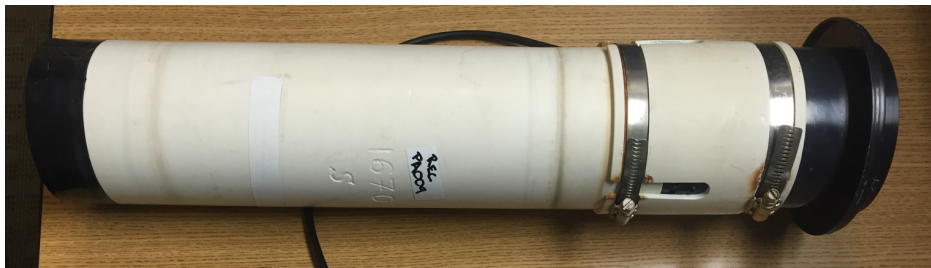
Figure 8: TFlex rain gauge with broken top funnel (right).
