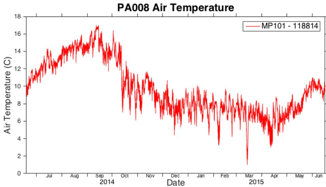
Figure C 6: Secondary (Flex MP101) air temperature sensor. Data were flagged Q4 from May 7<sup>th</sup>, 2015 to the end due to diverging temperature measurements.
