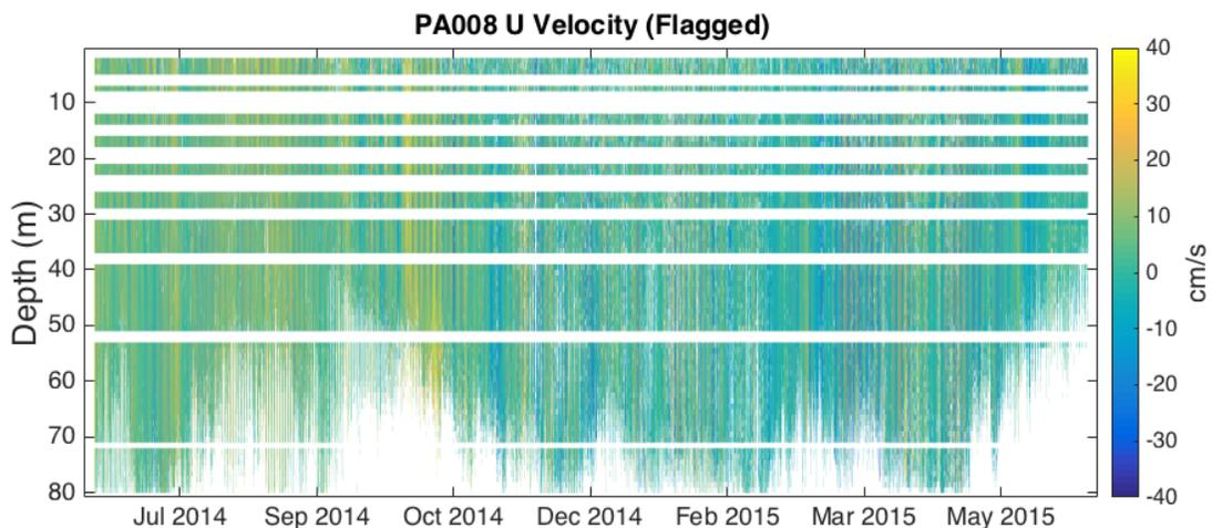
Figure 14: ADCP eastward velocities with manual flagging thresholds and bin-flagging applied, in addition to the autonomous flagging thresholds applied by the ADCP. All interference caused by instruments on the mooring line is removed.
