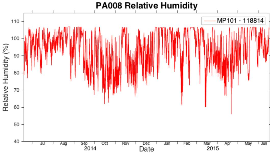
Figure C 5: Secondary (Flex MP101) relative humidity sensor. The entire record is flagged Q4 due to values over 100% in a time-series that was offset from the other ATRH sensors.
