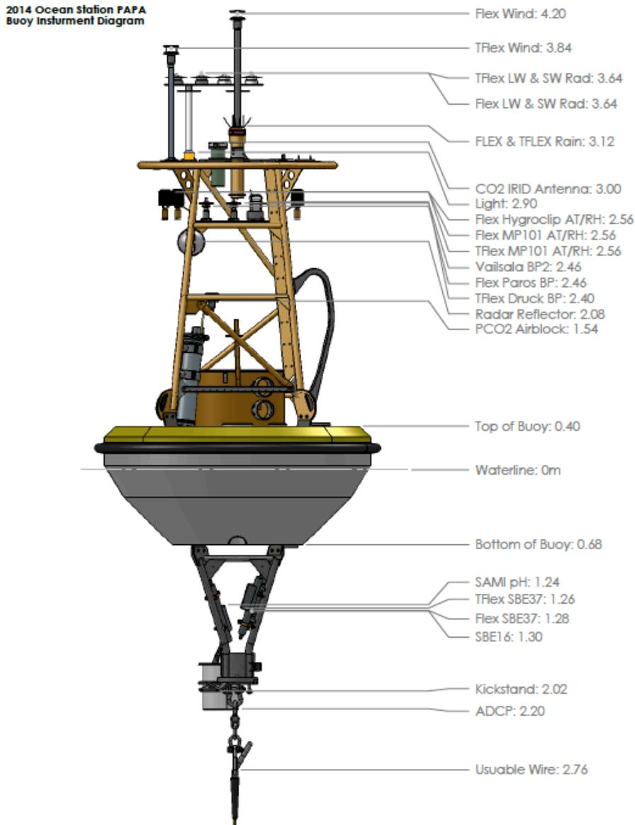
Figure 4: Buoy diagram showing bridle arrangement. The SBE16 package contains a suite of sensors.
