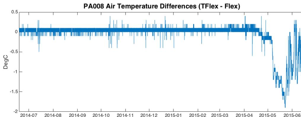
Figure 6: Air temperature time-series and difference plot from PA008. The TFlex drifts from the Flex and Hygroclip sensors in May (denoted by arrow), but occasionally returns to within 0.2°C.
