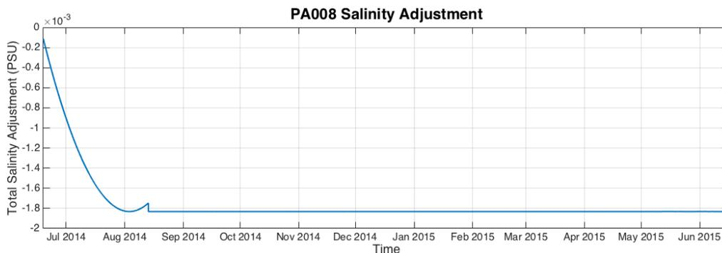
**Figure 12: Cumulative salinity adjustment (curve detrend + conductivity offset), starting from the average calibration. This plot represents the black minus magenta line in Figure 11.**
