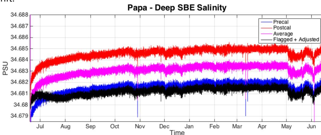
Figure 11: PA008 (2014 - 2015) deep Seabird salinity data with pre-deployment (blue) and post-recovery (red) calibration coefficients applied. Calibration variability, seen here as a vertical offset, and early deployment drift stand out against the signal, despite a compact y-axis. The average calibration (magenta) and final product after the offset continuity adjustment and flagging (black) are shown.
