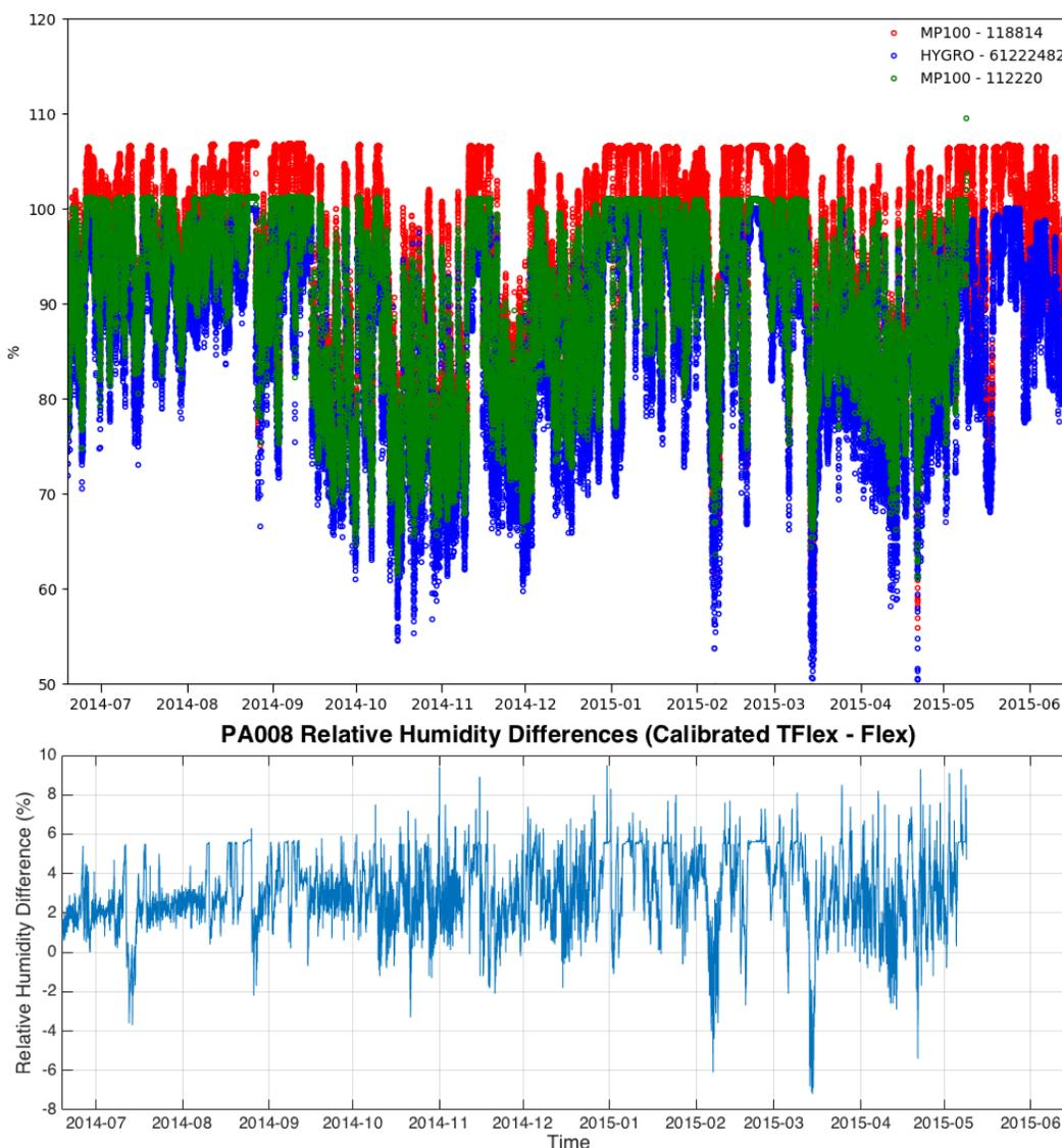
Figure 7: Relative humidity from the Flex (red) and TFlex (green) MP101s (upper), with difference plot (lower). The hygroclip (blue) is not considered a reliable field sensor, but is included for comparison.
