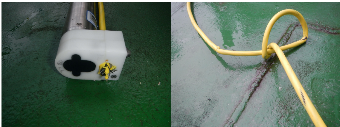
Figure 6: Nilspin break below S/N 7780 (left) and knot (right) on KE015a discovered during the redeployment cruise.
