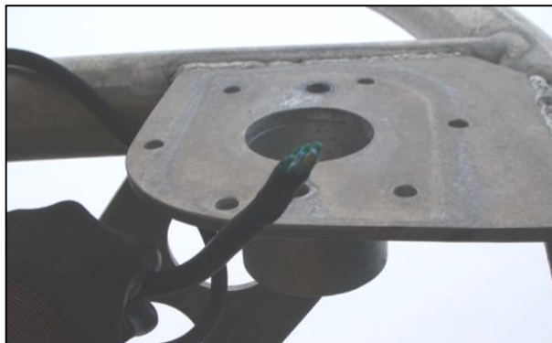
Figure 2: Sheared cable of missing Vaisala.
