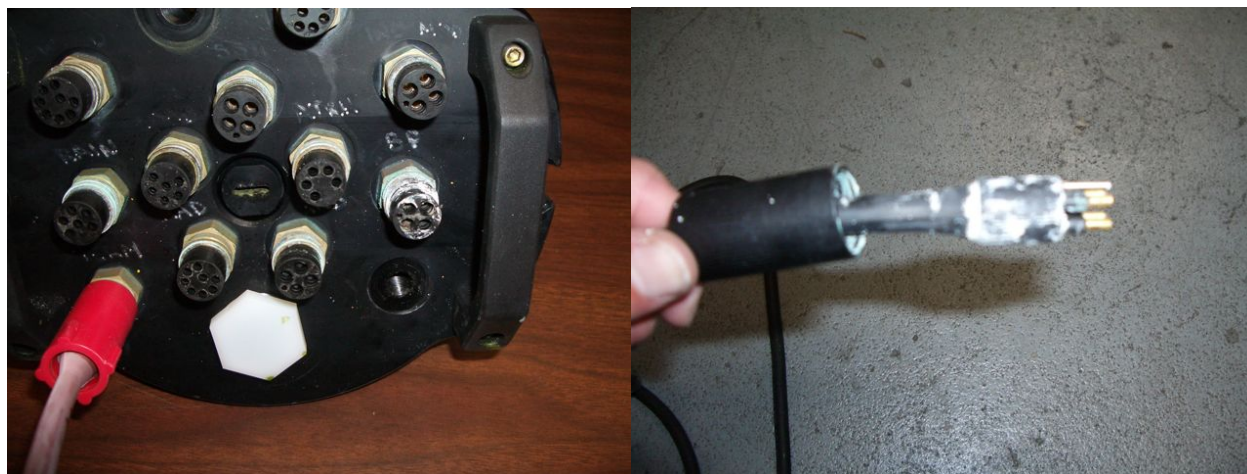
Figure 3: Corroded mating connectors of Paros barometric pressure sensor.
