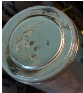
Figure 4. Broken Weld, Scorching
