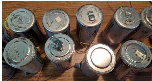
Figure 2. Broken Tabs & Welds
