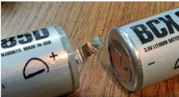
Figure 1. Broken Tab Between Cells
