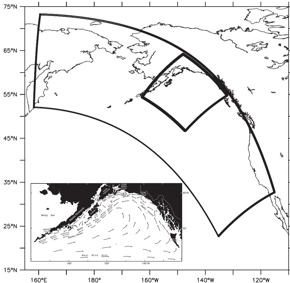
**Fig. 1.** Diagram of the nested model grids. The two grids of interest are NEP (large box, 10 km), and CGOA (small box, 3 km). Inset is map of the Coastal Gulf of Alaska with its major current systems.
