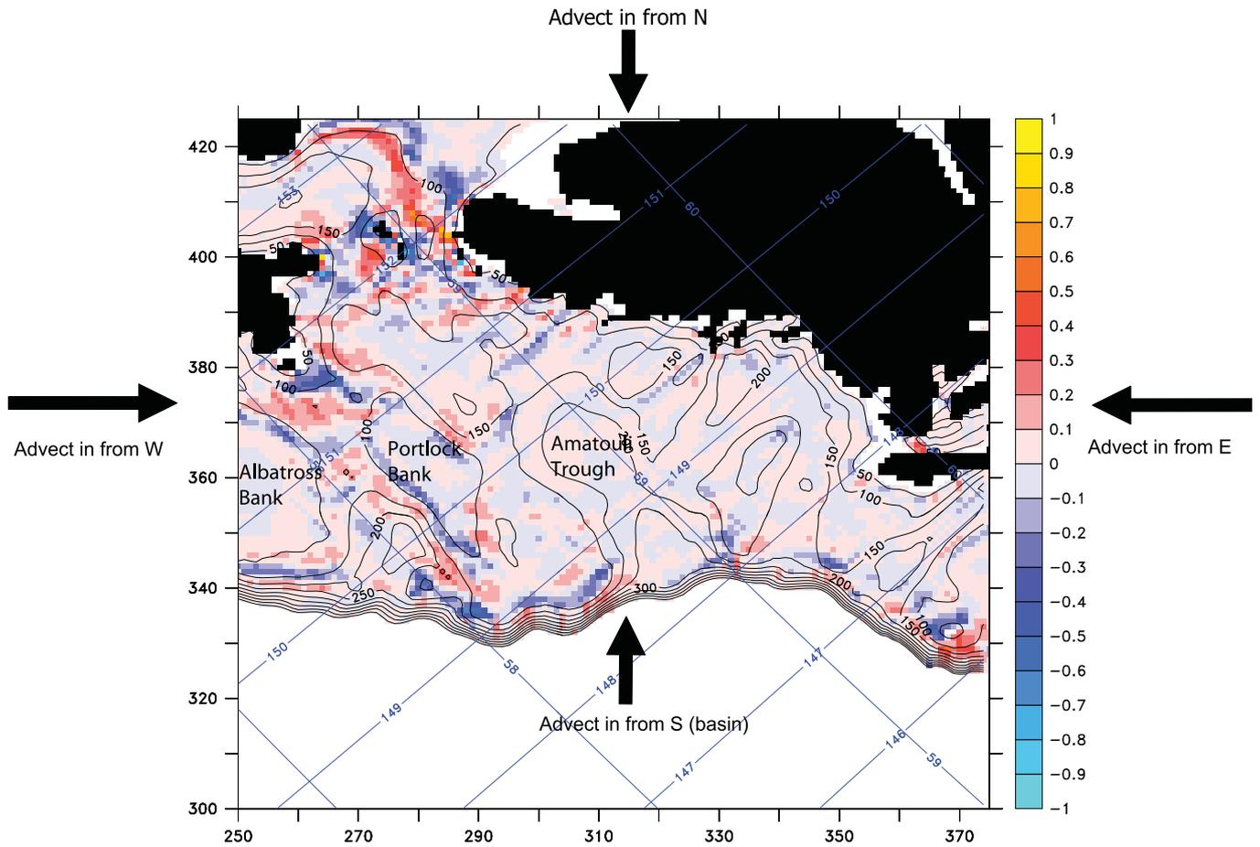
**Fig. 8.** Control volume used in water and nutrient flux calculations. Calculated monthly average vertical flux of water ( $\text{mm s}^{-1}$ ) through the 15-m-depth horizon for May 2001 is shaded. Positive/negative values indicate upward/downward flux. In this and subsequent spatial maps, the x- and y-axis are in native model coordinates with grid spacing  $\sim 3$  km. Also shown here are bathymetry (black lines) and the latitude-longitude grid (blue lines).
