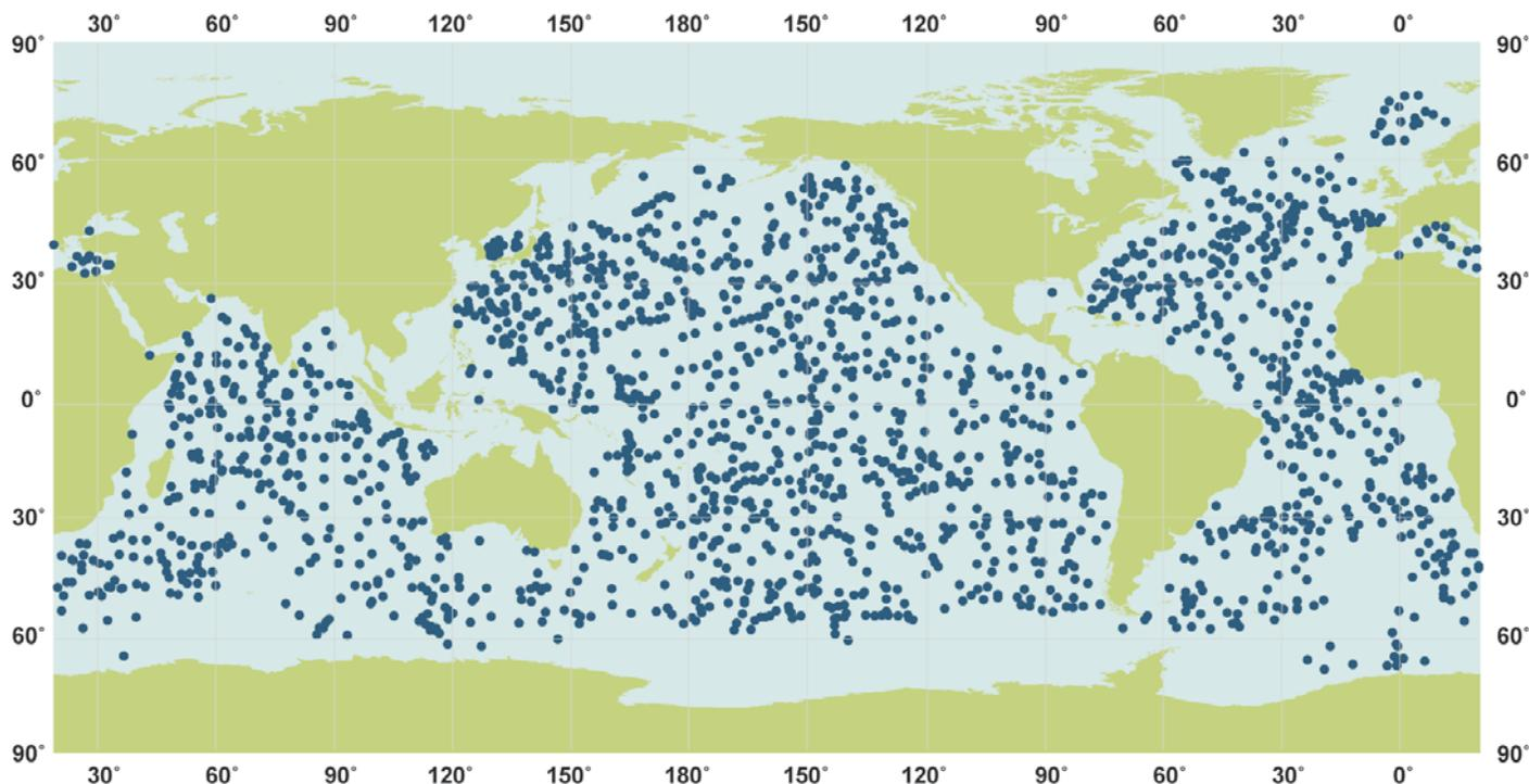
*Locations of Argo floats, which provide a new source of data from the top 2 km of the ocean. There were 1894 active floats as of June 13, 2005. The robotic floats spend most of their lives at depth but surface regularly to make temperature and salinity profile measurements. Many countries contribute the floats, and all data are freely available. A challenge for the Argo program will be the deployment of floats in Arctic waters. NOAA funds the U.S. Argo component.*
