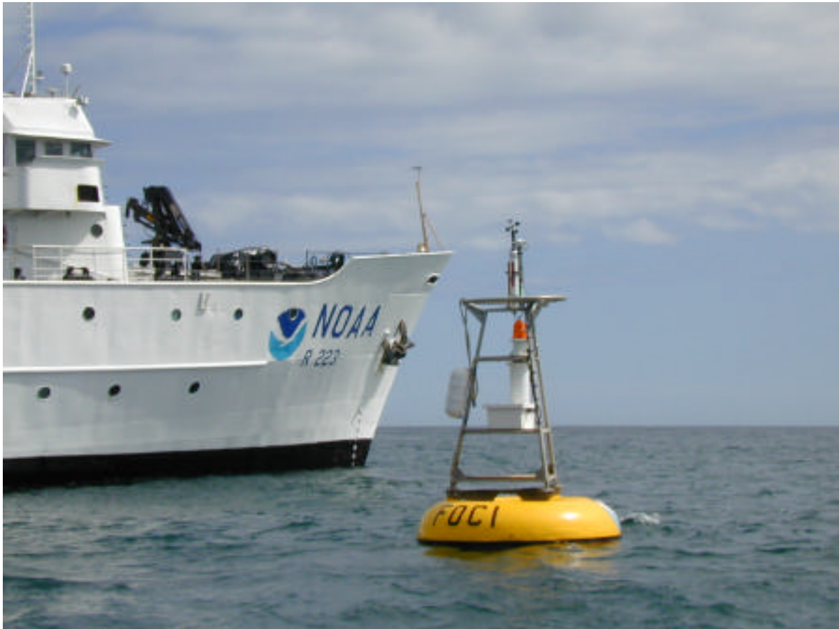
Figure 3. Photograph of surface float of BSM-2 (FOCI-Peggy).
