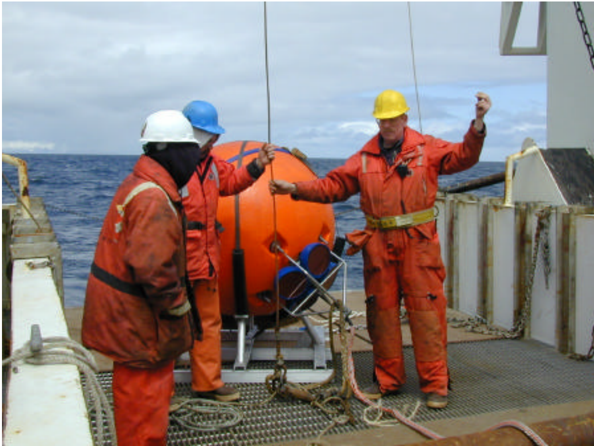
Figure 4. Photograph of syntactic float with ADCP.
