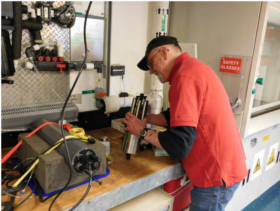
Dean Stockwell cleaning the uncontaminated seawater optical sensor suite. The ISUS for underway nitrate samples is shown strapped to the bench on the left. Prior to our arrival marine technicians Ethan Roth and Steve Roberts had integrated the data stream into the ship's continuous underway sampling suite.
