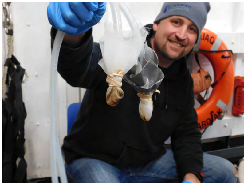
Filters clogged with algae at DB03.8.
