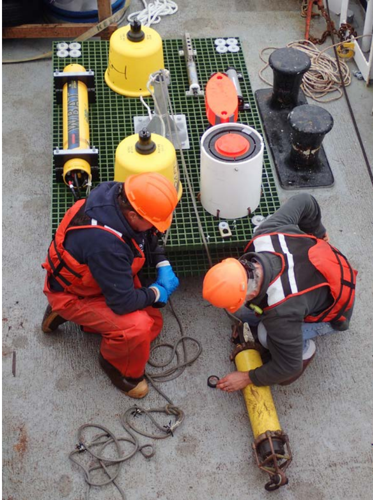
Setting up fish acoustics mooring for deployment (J. Vollenweider)
