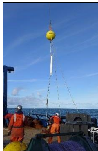
Figure 2. Long-term passive acoustic mooring being deployed.
