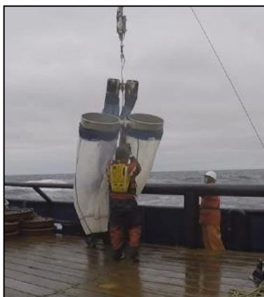
Figure 23. Bongo nets being deployed.
