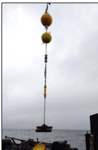
Figure 11. Oceanographic ADCP mooring being deployed.
