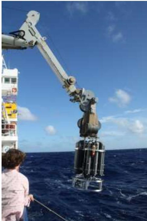
CTD instrument deployed from R/V Revelle.
