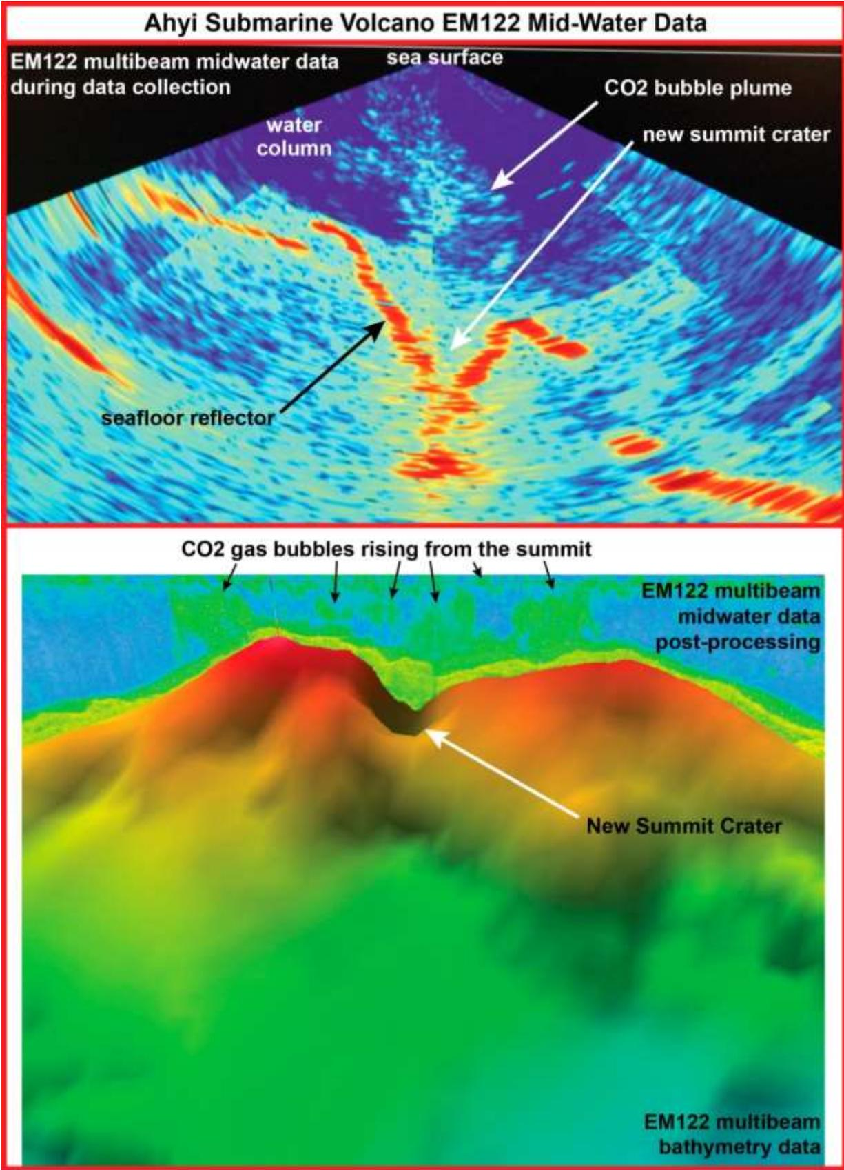
Figure 4.5-3. EM122 mid-water data collected on RR1413 at Ahya seamount. Top image shows seafloor and midwater data during collection, the bottom image shows the data post-processed. The new crater created by the April 2014 eruption is visible in both images, as well as the CO<sub>2</sub> bubbles rising from the summit.
