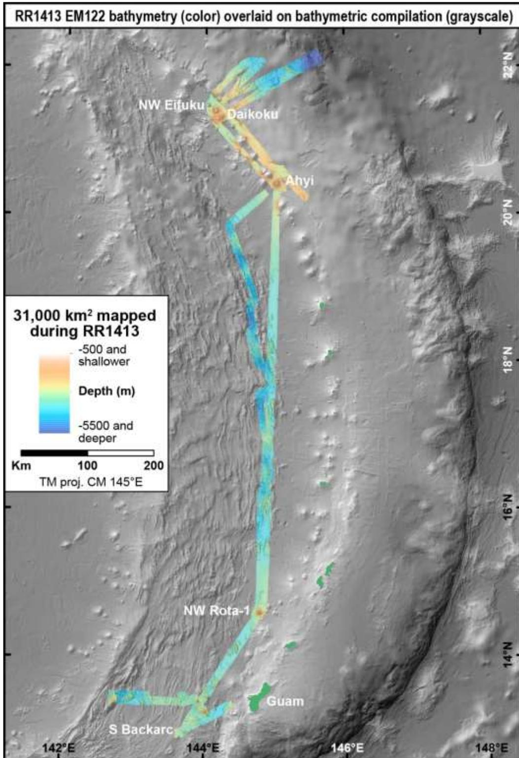
Figure 4.5-1. RR1413 EM122 bathymetry data (color data) overlaid on previous bathymetric compilation (grayscale), showing the 31,000 km<sup>2</sup> mapped during the expedition.
