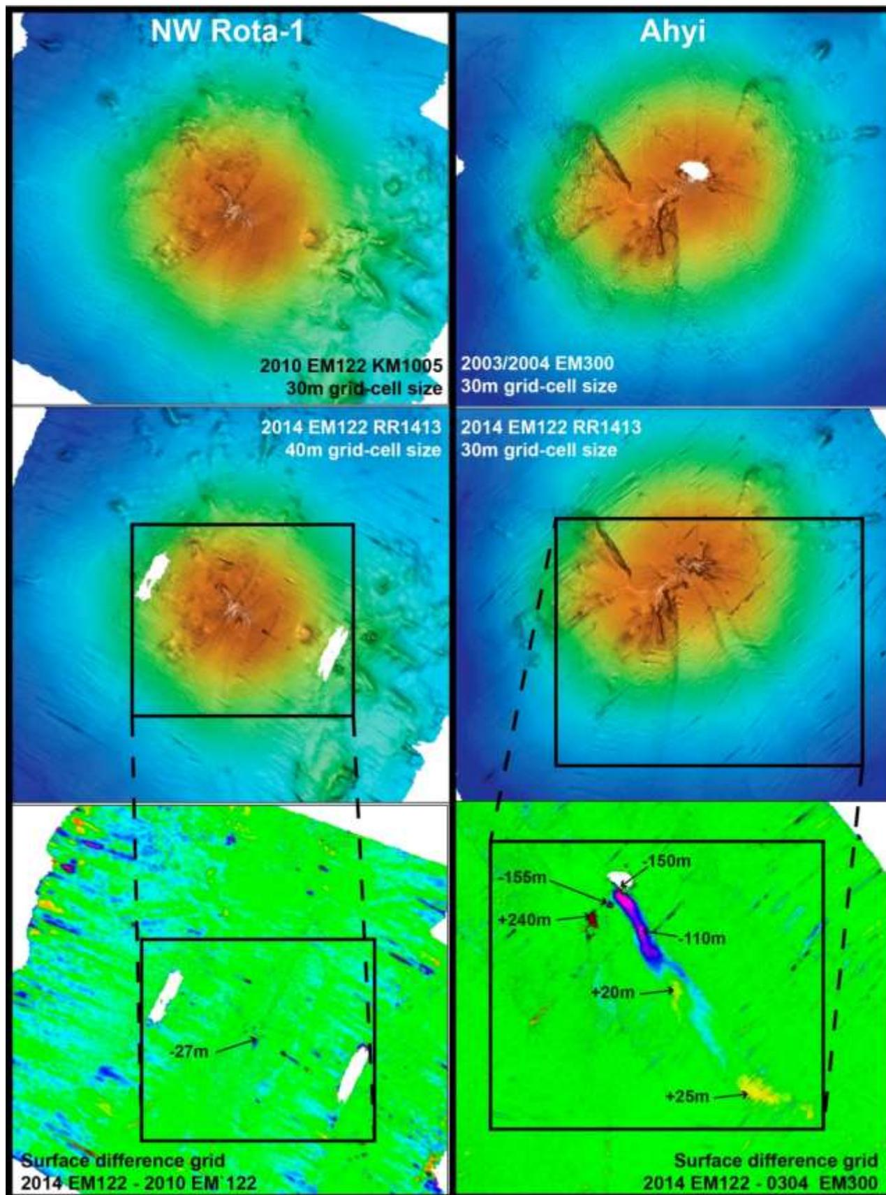
Figure 4.5-2. Bathymetric comparisons showing depth changes at NW Rota-1 (left) and Ahyi (right). EM122 data from the RR1413 expedition were compared to previous surveys to create the surface difference grids at the bottom of the figure.
