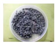
Figure 4.1.1-4 S34-Bio-09 Sulfur tadpoles, globules and Pele's tears.
