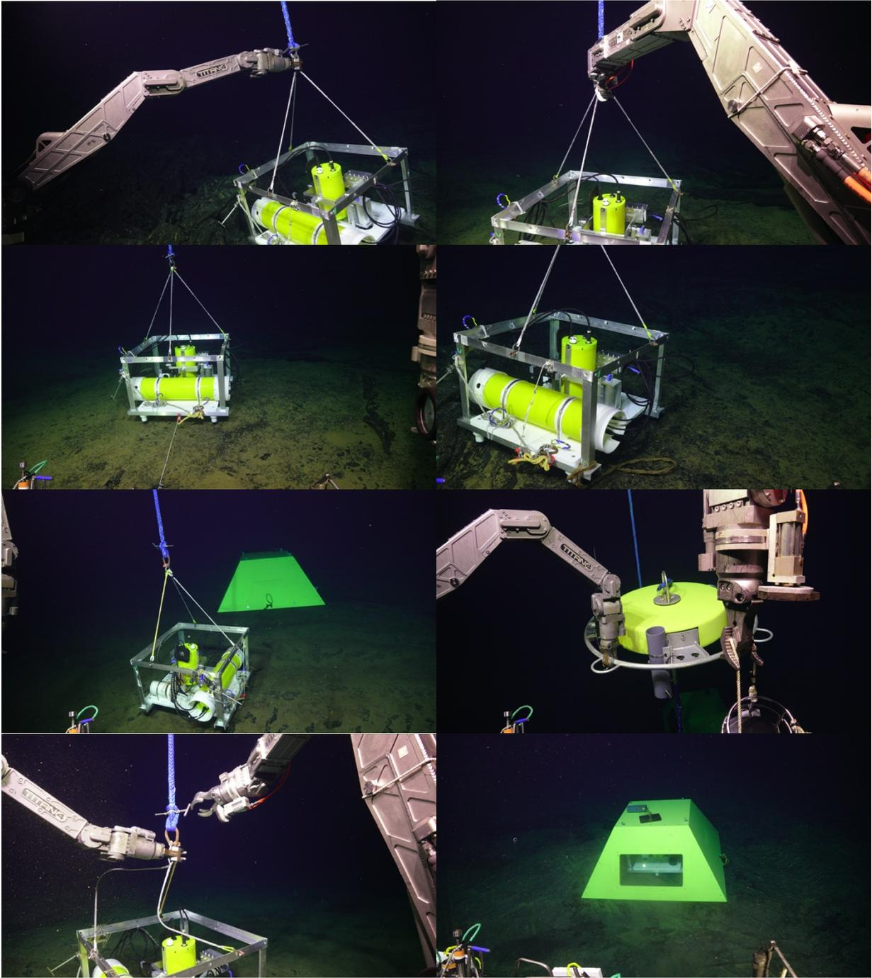
Figure 4.5.2 - ROV Jason images of the Webb Crustal Compliance instruments being deployed on the seafloor.
