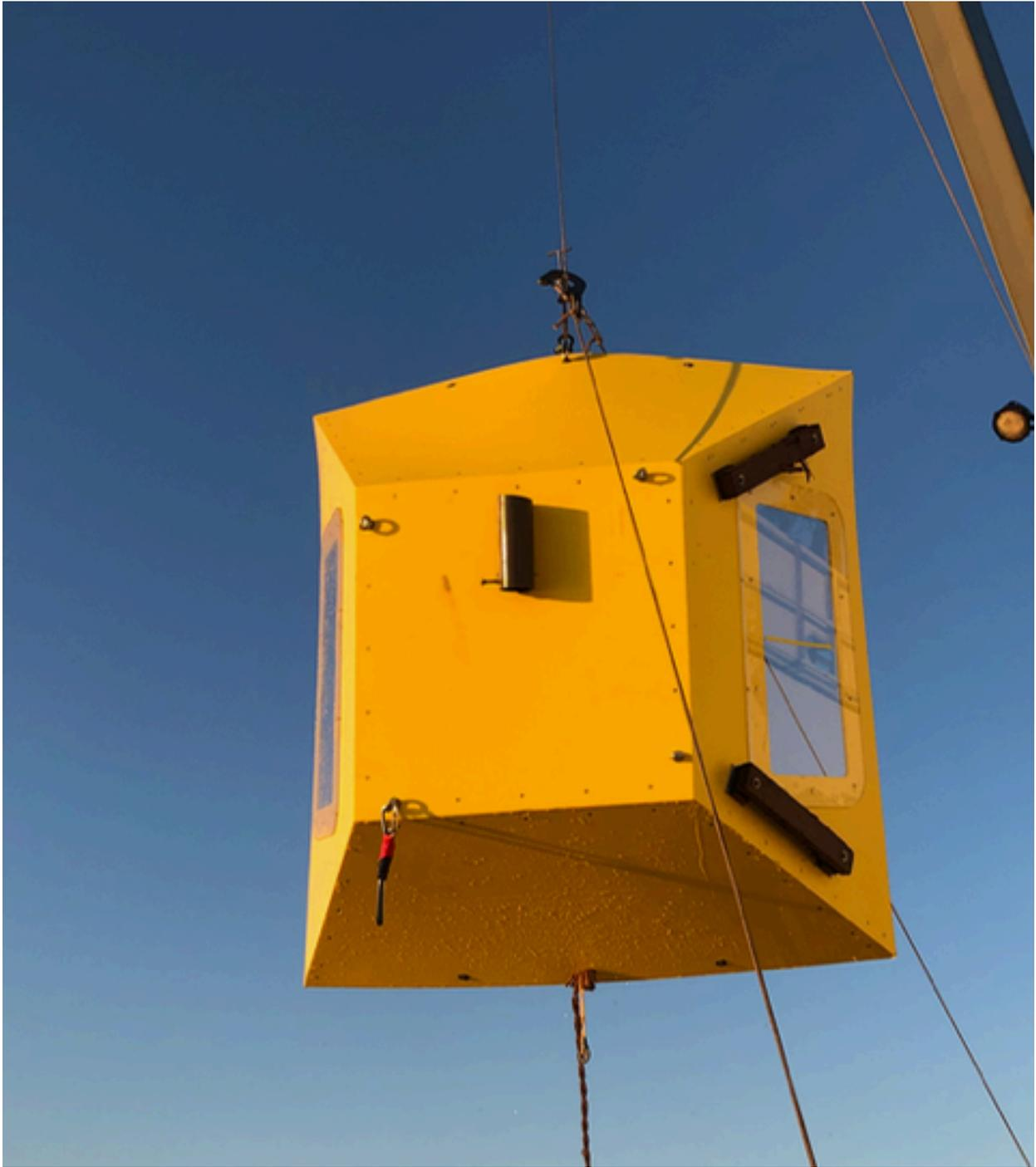
Shield coming out of water. Note Jason hook in eye at top (as well as a tag line hook). Line to instrument base is hanging down. Is the shield without the extra S/S plate along edge? (on we added Jason weight added somewhere- do we need to replace this with a S/S plate on third one?)
