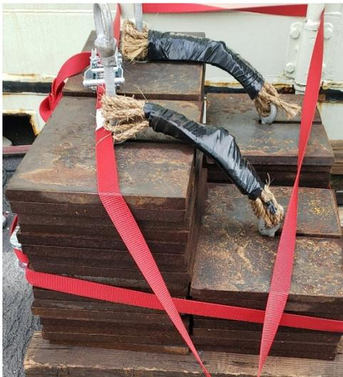
Drop weight stack for float pack counted 25 plates per deployment (24 x 15lbs = 360lbs).
