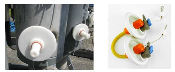
• Fill sample bottle—Attach the designated end of the Tygon tubing to the stopcock/petcock of the water sampler. Insert Tygon tubing to the bottom of the sample bottle, open air valve, open water valve, and begin water flow. Invert the bottle over the tube to rinse the bottle carefully with the sample water, moving
