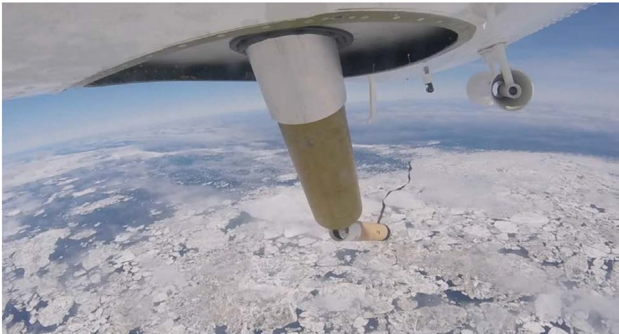
Fig. S2. Airborne Expendable (AX) launch chute on NOAA 56, during the deployment of an atmospheric dropsonde.
