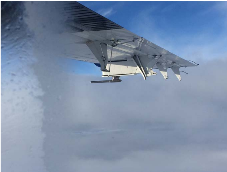
Fig. S1. ARIM200 Air Data Probe mounted on the pylon on the right wing of NOAA 56.
