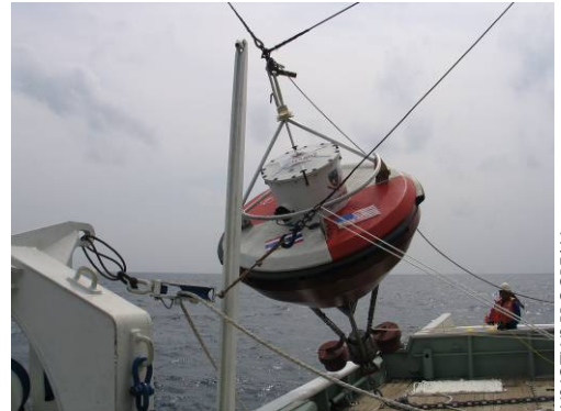
Technician lowers the DART tsunami detection buoy into the waters off of Phuket, Thailand.
