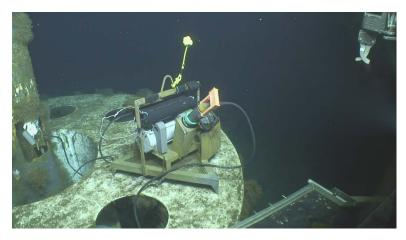
Figure 104  $\,8/25/2012\,$  (RGB.20120825\_055712\_733) CORK 1025 showing CORK logger being interrogated using an ODI connection to the ROV.
