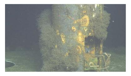
Figure 102 8/25/2012 (RGB.20120825\_043159\_864) CORK 1025 showing pressure connection prior to attempting to hook up .
