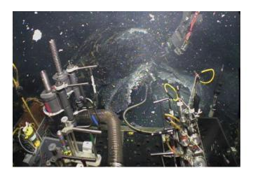
Figure 66 Boca vent. HFS nozzle in the opening, taking fluid samples. 23:49 8/20/2012.
