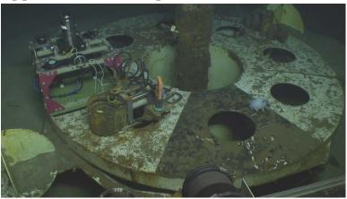
Figure 96 8/24/2012 (RGB.20120824\_083255\_505) CORK 857D showing the optical modem (left) and the 'new' CORK logger to the right of the optical modem. An ODI UWMC connects the new logger with the optical modem. The'old' CORK logger is seen to the rear of the CORK platform.
