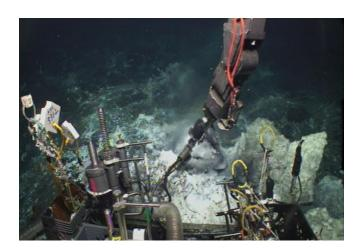
Figure 90 sampling hot fluid at Vixen vent, T by HFS 345.3, with Jason probe 352. Observed flashing/emulsion in fluid indicative of boiling. Heading 334, depth 1534. Took 2 piston samples here. The HOBO T recorder was not visible in this vent and may have been buried. HOBO recorder was still visible in nearby Casper.
