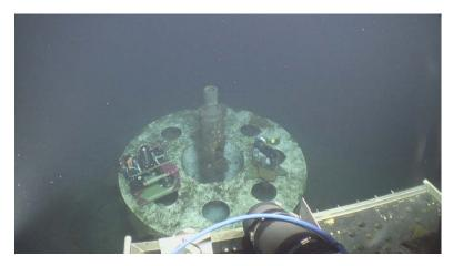
Figure 101 8/25/2012 (RGB.20120825\_042919\_172) CORK 1025 with optical lander (left) and cork logger (right).
