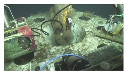
Figure 103  $\,8/25/2012$  (RGB.20120825\_052942\_810) CORK 1025 showing pressure connection hooked up to CORK logger and logger connected to the optical modem.
