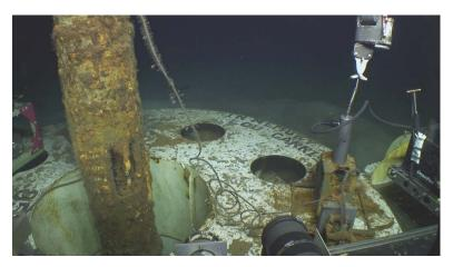
Figure 97  $\,8/24/2012$  (RGB.20120824\_091245\_445) connecting to the old logger using the SeaCon UWMC, CORK 857D.
