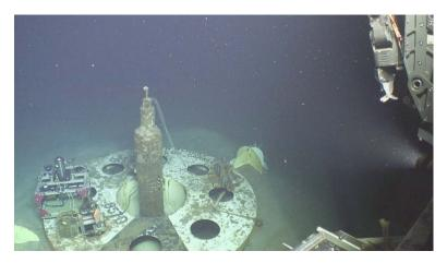
Figure 100 8/24/2012 (RGB.20120824\_123934\_904) CORK 857D with optical lander and new cork logger (left) and old cork logger (right).
