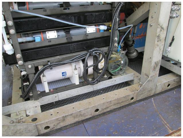
Figure 6 HFPS in aft starboard corner of Jason. Large volume bag sampler is the clear plastic cylinder with metal handle and green tape forward of HFPS.
