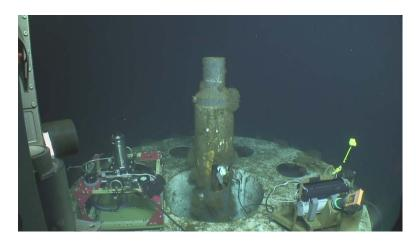
Figure 105 8/25/2012 (RGB.20120825\_055842\_722) CORK 1025 showing final configuration of CORK logger (right) and optical modem (left).
