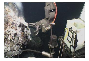
Figure 27 Attempt to grab sulfide chimney from Hell. Friable chimney crumbled (same result as Inferno).
