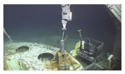
Figure 98  $\,$  8/24/2012 (RGB.20120824\_092305\_428) connecting to the old logger using the SeaCon UWMC, CORK 857D.
