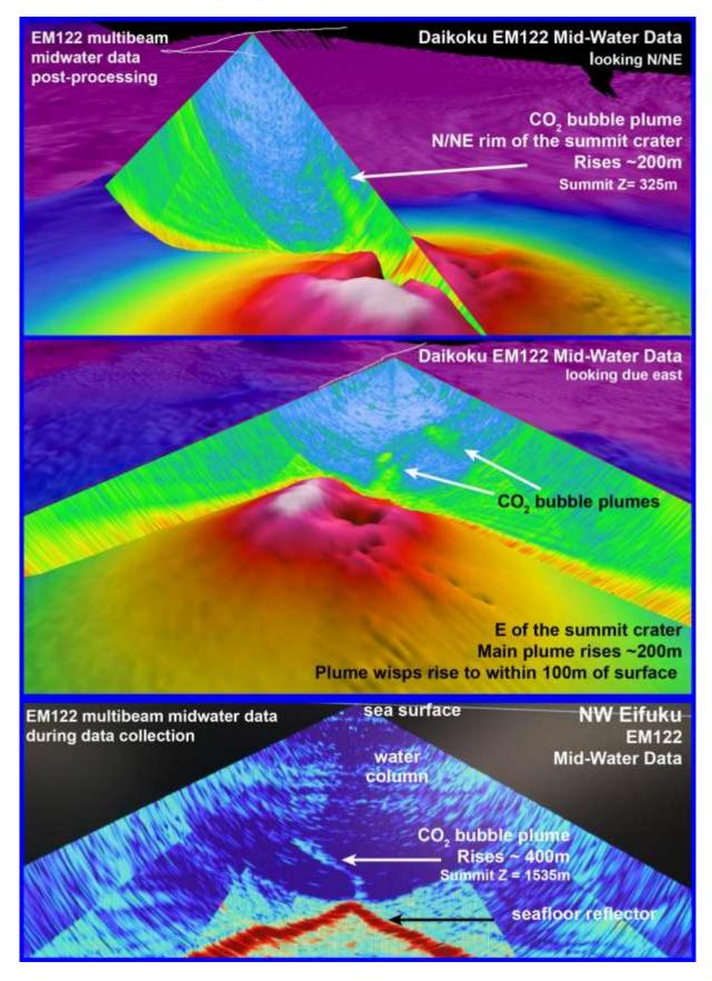
Figure 4.5-6. (a, b) Processed mid-water data at Daikoku showing the 2 separate areas of venting at/near the summit. c) NW Eifuku midwater data during collection. The CO2 bubble plume can be seen ascending from the summit area.
