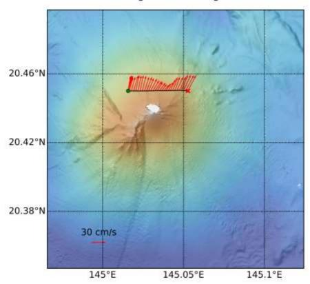
**Figure 4.3.2-1**. CTD tow transect for Ahyi towyo T14B-01. The green dot and red X represent the transect beginning and ending points, respectively. The red arrows represent average current direction and magnitude over observed plume depths, in this case 50 to 170 meters.
