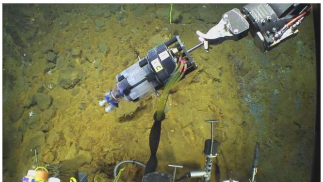
BioMat cassette sampler with ferrozine at NW Eifuku, J2-799.
