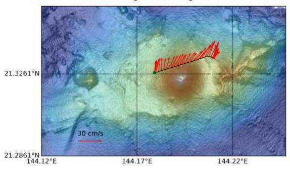
**Figure 4.3.2-2**. CTD tow transect for Daikoku towyo T14B-03. The green dot and red X represent the transect beginning and ending points, respectively. The red arrows represent average current direction and magnitude over observed plume depths, in this case 300 to 450 meters.
