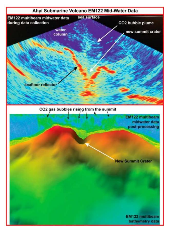
Figure 4.5-3. EM122 mid-water data collected on RR1413 at Ahyi seamount. Top image shows seafloor and midwater data during collection, the bottom image shows the data post-processed. The new crater created by the April 2014 eruption is visible in both images, as well as the CO<sub>2</sub> bubbles rising from the summit.
