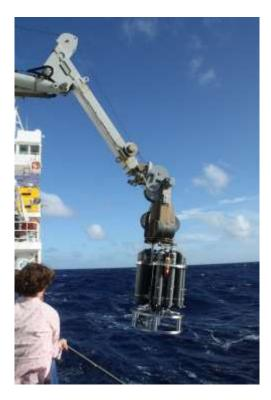
CTD instrument deployed from R/V Revelle.
