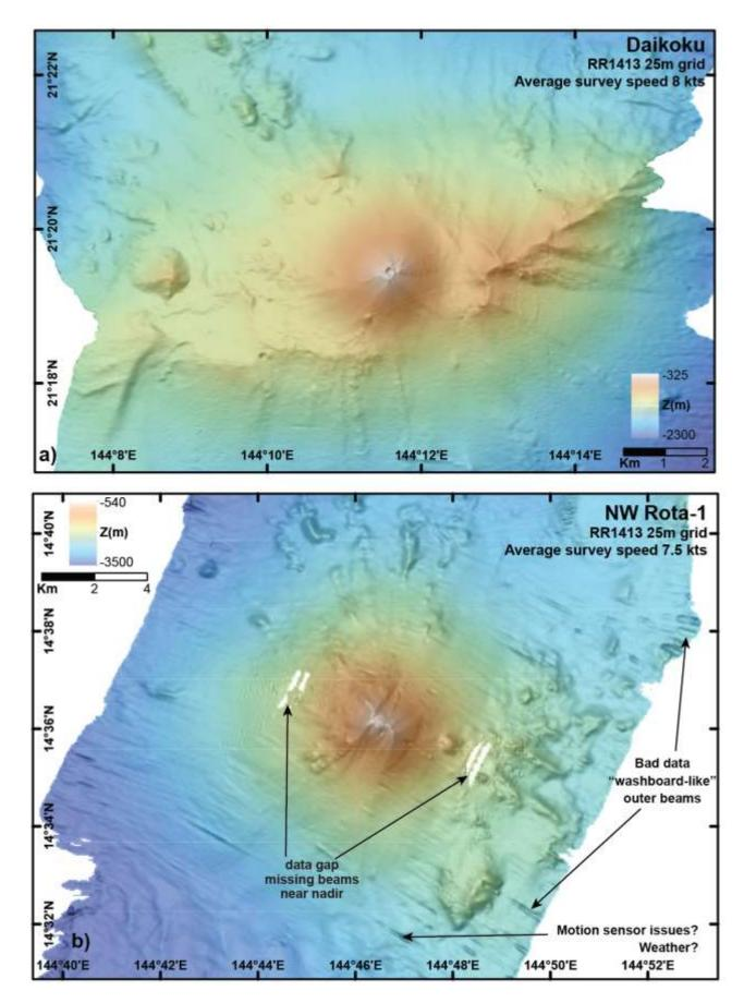
Figure 4.5-5. (a) The entire bathymetric survey at Daikoku. (b) The entire bathymetric survey at NW Rota-1, highlighting some of the bathymetric data quality problems encountered on the expedition.
