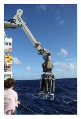
CTD instrument deployed from R/V Revelle.
