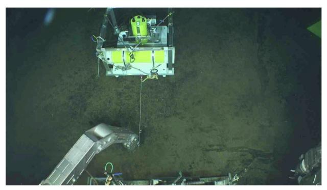
Jason pulling out fiducial line. Need to make point where Jason drops edge of shield a little easier to see, but otherwise this seems to work well.
