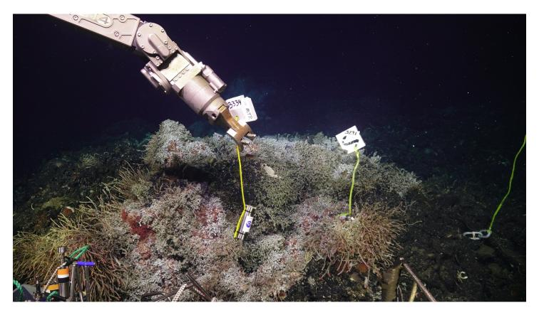
Placing MTR temperature recorders at Anemone vent in the ASHES vent field on ROV Jason dive J2-1293.
