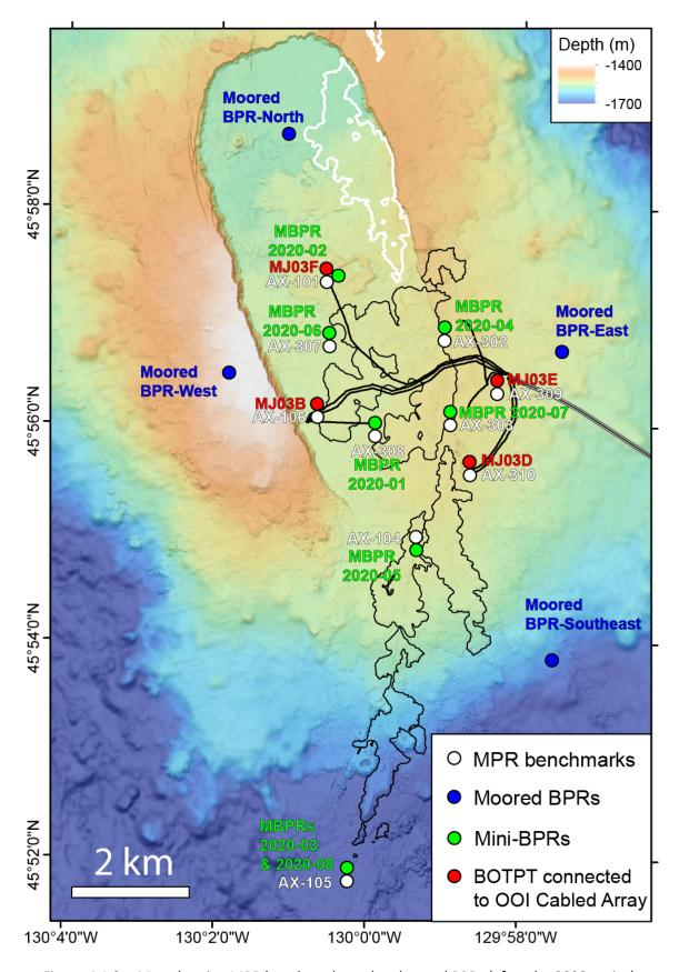
Figure 4.1.2. - Map showing MPR benchmarks and co-located BPRs (after the 2020 cruise).
