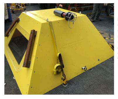
Shield pre-deployment with USBL beacon. Need to change front bars to something that doesn't get destroyed by Jason arms. Extra Jason weight attached to eye on panel on back side to speed fall (not visible). Eye for hook from instrument base to shield is on right front panel edge- need to consider changing that to make it easier for Jason to hook in to (so it doesn't flop around as it tried to hook- use U bolt?).
