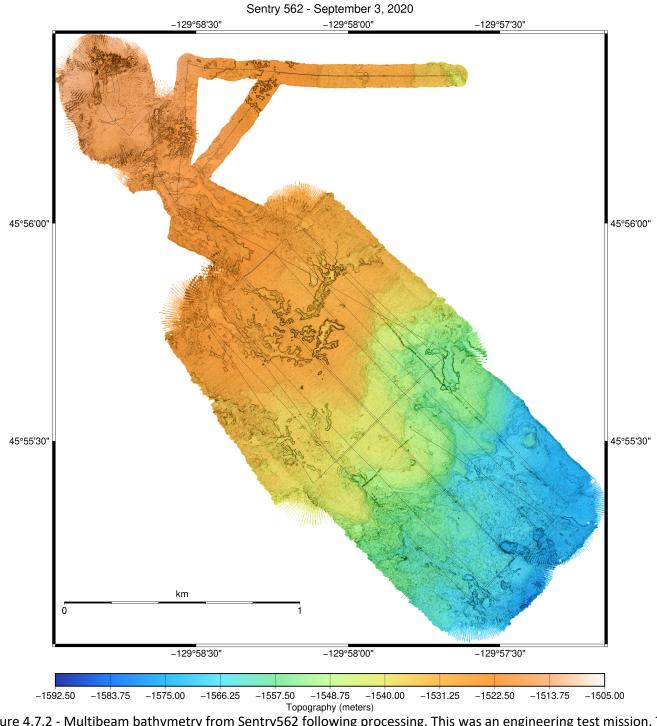
Figure 4.7.2 - Multibeam bathymetry from Sentry562 following processing. This was an engineering test mission. The speed of sound value used for beamforming was incorrect, but this has been corrected in post processing.
