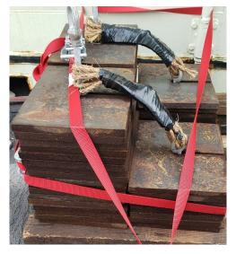
Drop weight stack for float pack counted 25 plates per deployment  $(24 \times 15 \text{lbs} = 360 \text{lbs})$ .
