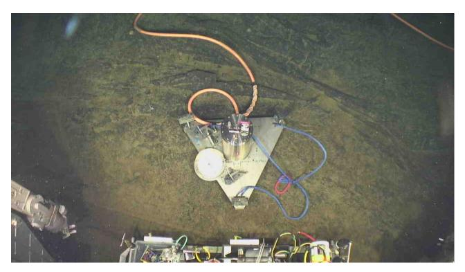
• The second and third images below (04:34:06 & 04:36:06) are before and after PilotCam views of the move we made with the SCTA. The ROV was on the bottom with a heading of 175, and did not move while we lifted the SCTA and repositioned it to the right. There was a slight rotation of the SCTA during the move, but nowhere near 110°.
