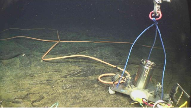
• The fourth image below (05:04:06) is after the move & leveling from the BrowCam with an ROV heading of 161° (appended to the file name). This shows that the SCTA was rotated something like 10-20° during the move and that in the new orientation the -X direction is about 160° or perhaps a little less.
