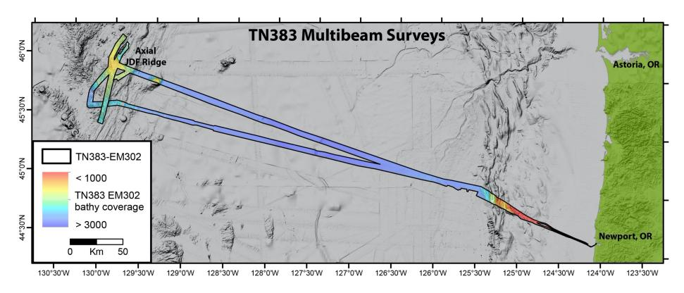
Figure 4.10.1 – Map of EM302 multibeam data collected during TN383.
