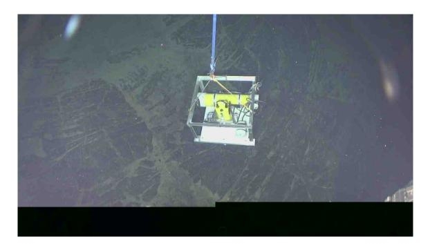
Instrument hanging from float on nice sheet flows. Two extra weights to speed fall were removed before float pack & instrument were moved into position.
