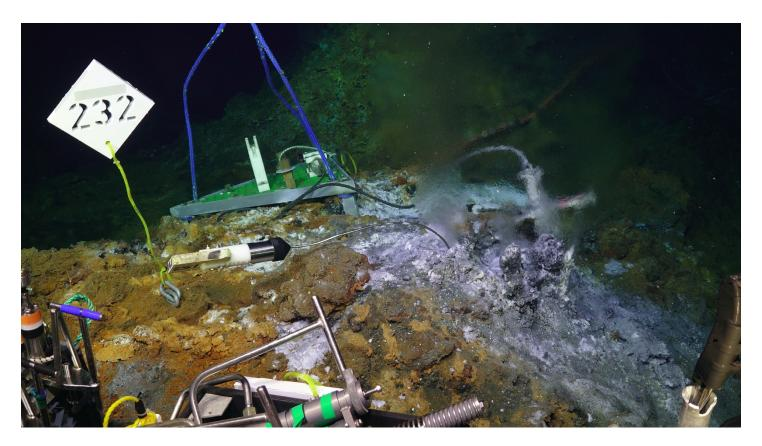
New HOBO temperature probe and marker 232 at Diva vent in the International District vent field seen on ROV Jason dive J2-1296.
