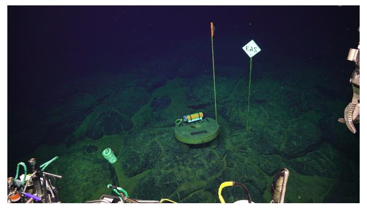
Approach to pressure benchmark AX-101 at the center of the caldera during ROV Jason dive J2-1295. A mini-BPR is already on the benchmark. White bucket to the left is a tephra sampler.
