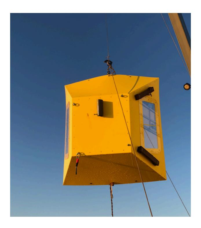
Shield coming out of water. Note Jason hook in eye at top (as well as a tag line hook). Line to instrument base is hanging down. Is the shield without the extra S/S plate along edge? (on we added Jason weight added somewhere- do we need to replace this with a S/S plate on third one?)
