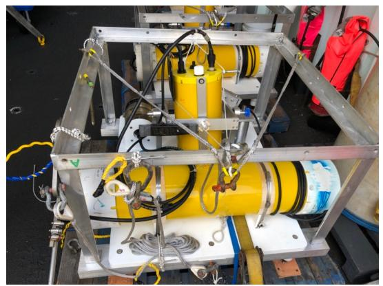
Instrument ready for deployment. Line to shield held in place by shock card with pull pin on upper bar. Hook held to frame with leftmost pull pin. Short fiducial line with shackle at end to allow alignment of shield over instrument base is lower pull pin. Harness is draped on top.
