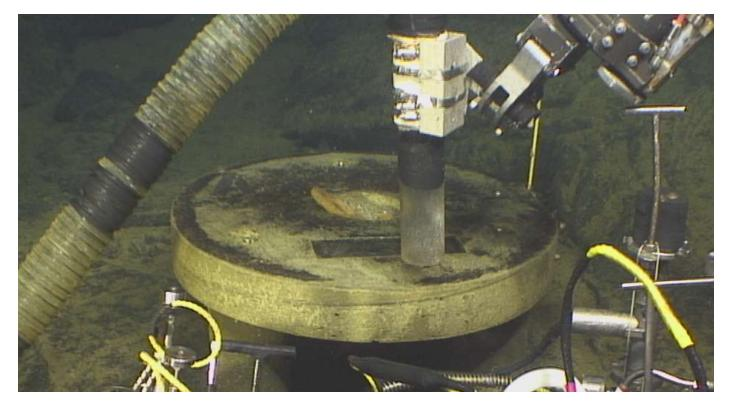
**Figure 4.1.2-5** Framegrab of sample J823-Geo-01 being collected from the pressure measurement benchmark AX-101 in the central caldera. The suction sampler held in the manipulator is vacuuming the black particles of volcanic glass (ash), which was mostly limu o Pele, that had settled on the benchmark.
