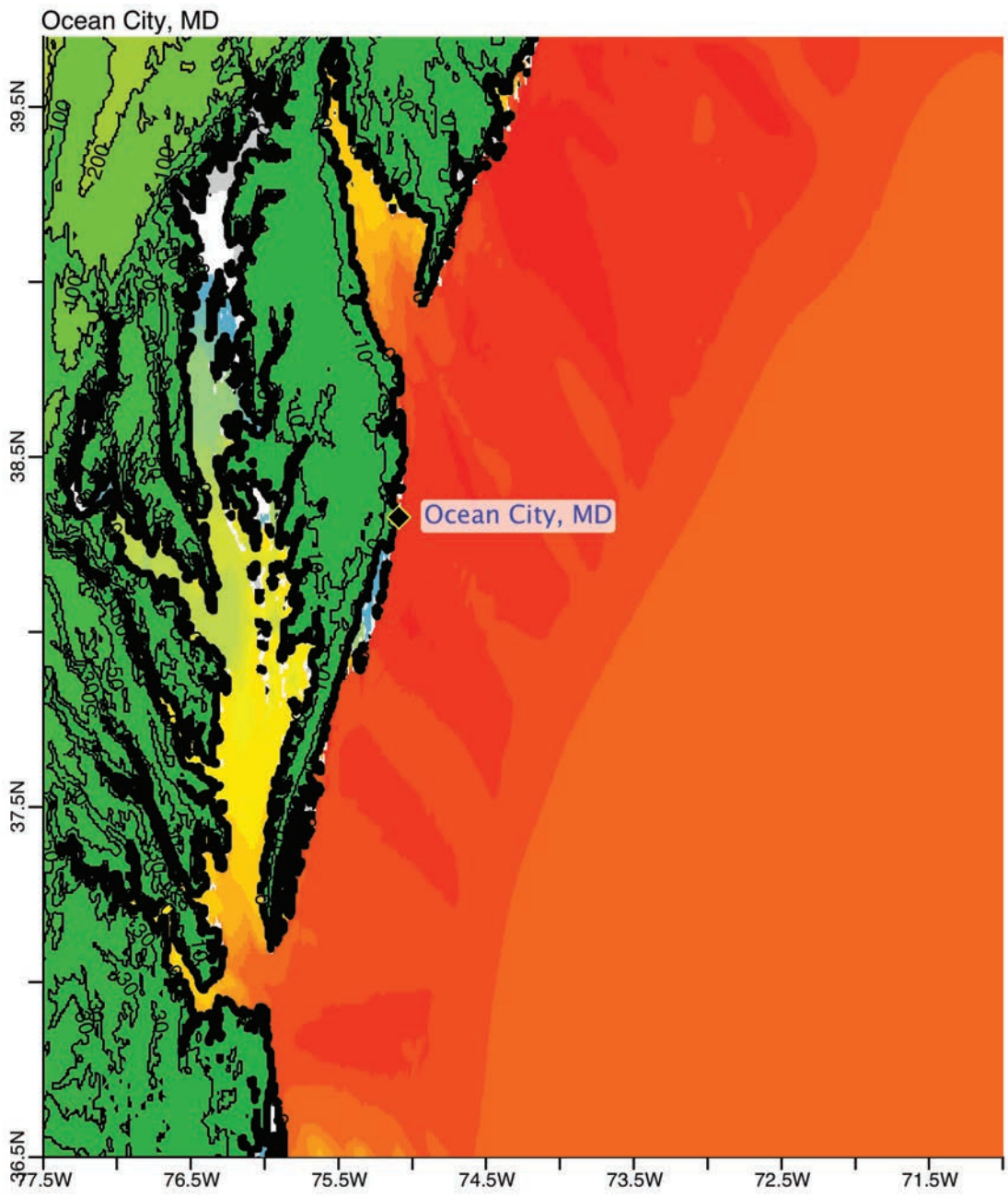
Figure 5. Max computed wave amplitude of A grid, Ocean City, Maryland, for synthetic event ATSZ 48-57.
