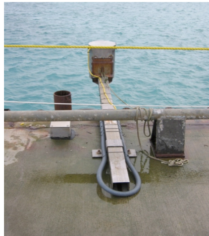
Figure 6 Images of the Shemya tide gauge and its installation on the Alcan pier on the northwestern side of the island.
