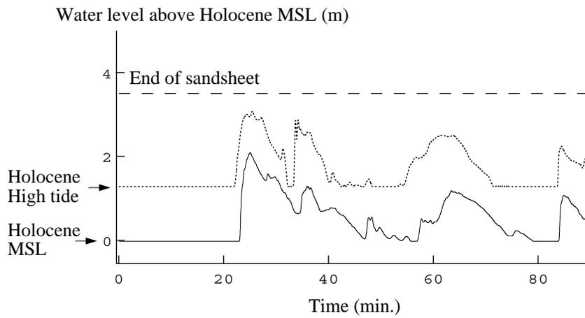
Figure 7: Computed tsunami waveforms at the western head of Cultus Bay.
