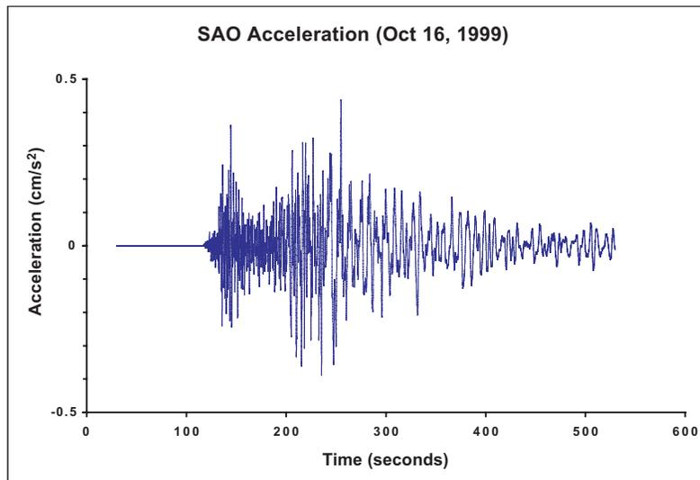
**Figure 3:** Time series of the vertical acceleration produced by the 16 October 1999 Hector Mine earthquake in Southeastern California, as observed at the broadband San Andreas Observatory (SAO) seismic station.
