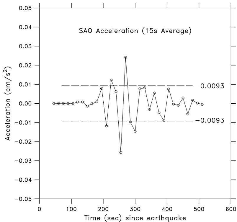
**Figure 4:** Vertical acceleration (15-second average) produced by the 16 October 1999 Hector Mine earthquake in Southeastern California, as observed at the broadband San Andreas Observatory (SAO) seismic station. Also shown are the threshold values needed to set the D123 DART station into tsunami event mode.
