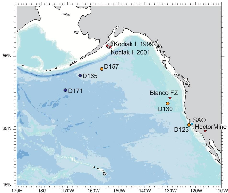
**Figure 1:** Map of the Northeast Pacific Ocean showing DART stations, the SAO seismic station (square) and the epicenters of earthquakes (stars) that have set DART systems into tsunami event mode. These DART systems (dots) are indicated in orange while other DART systems, presenting in place, are shown in blue.
