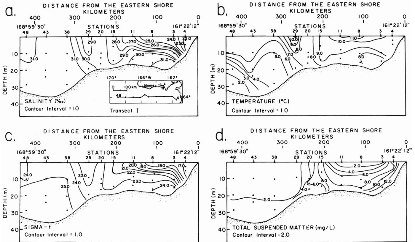
Figure 20-6. Vertical cross section of the distribution of: (a) salinity (b) temperature (c) sigma-t (d) total suspended matter for transect I in Norton Sound.
