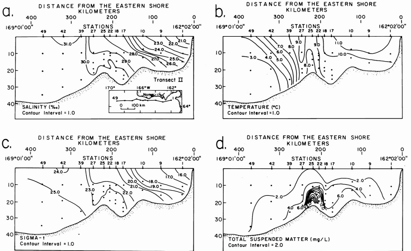
Figure 20-7 Vertical cross section of the distribution of: (a) salinity (b) temperature (c) sigma-t (d) total suspended matter for Transect II in Norton Sound.
