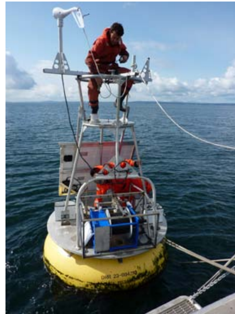
Colin Smith, UW ORCA buoy technician, works to service weather sensors on the profiling buoy off Pt. Wells in the Main Basin of Puget Sound. These buoys are solar powered and utilize a winch (blue box) to lower a water sensor package for temperature, salinity, oxygen, chlorophyll and other variables. Data are relayed in near real-time. Photo credit: Allan Devol
