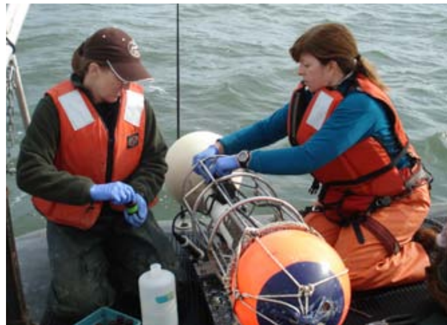
Suzan Pool (left) and Julia Bos (right) of Ecology's Marine Monitoring Unit deploying a serviced sensor package moored to a channel marker. Photo credit: Ecology's Marine Monitoring Unit.
