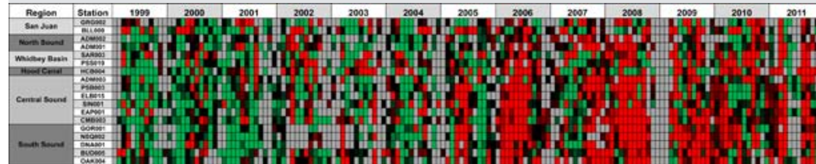
Figure 17. Monthly variability in nitrate concentration for stations in Puget Sound from 1999–2011. A shift from a prevalence of green to red cells indicates significant nitrate increases over the last 10 years. Each cell represents a monthly median nitrate concentration for samples from 0, 10 and 30m depths. Anomalies are defined as falling outside the inter-quartile (25 th to 75 th percentile) range for site and seasonal specific historic data since 1999. Color indicates anomalies: red < IQR, green > IQR and black = expected (within IQR) values. Grey fields denote no data available.
