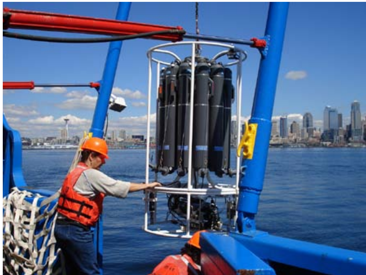
Jan Newton (UW, APL) retrieves a CTD-rosette sampling package at a station offshore from downtown Seattle during a PRISM cruise on Puget Sound on the EPA's Ocean Survey Vessel Bold in August 2008. Photo credit: Simone Alin, NOAA
