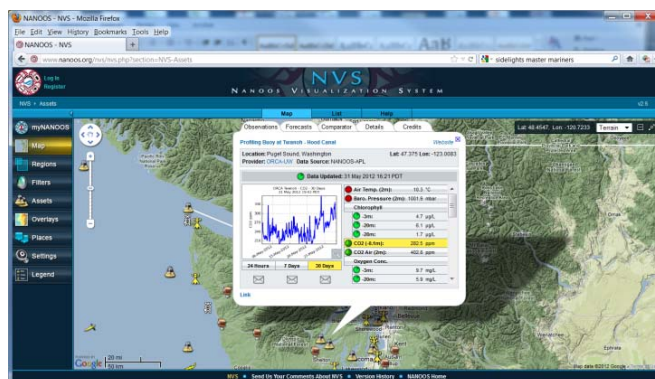
Fig. 1. Screen shot from NANOOS Visualization System showing 30 days pCO 2 data from a University of Washington buoy supported by NANOOS with NOAA PMEL sensors at Twanoh, Hood Canal, WA. The variation is being studied by scientists to understand underlying mechanisms driving OA in these local waters.
