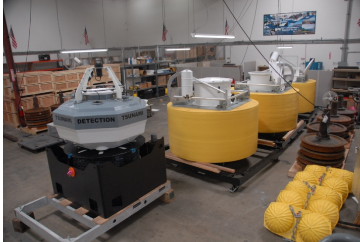
Fig. 2. Size comparison of ETD DART® system to STB.
