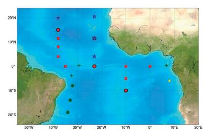
Fig. 1. The PIRATA backbone of ATLAS buoys (red squares), Northeast Extension (blue stars), Southwest Extension (green circles), Southeast Extension pilot project (yellow triangle), and island-based observation sites (green crosses). Buoys with barometers and the ability to estimate net heat flux are indicated with black circles.
