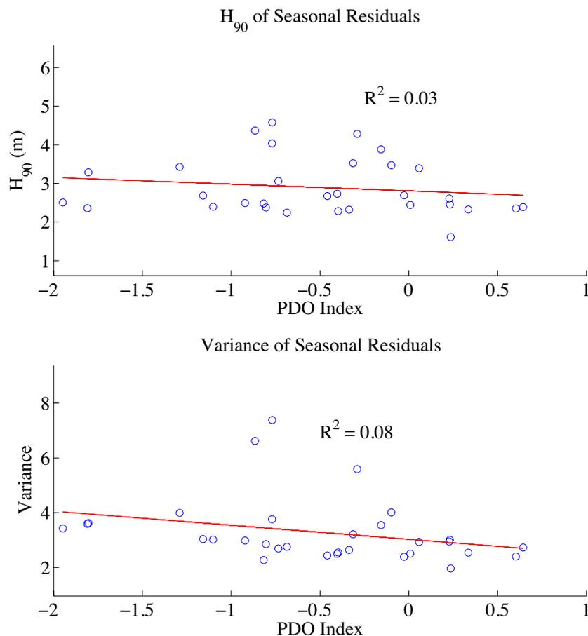
**Figure 8.**  $H_{90}$  and seasonal residual variance versus PDO index. In both cases, a weak dependence on PDO phase is demonstrated, though the dependence is stronger than observed in wind measurements.
