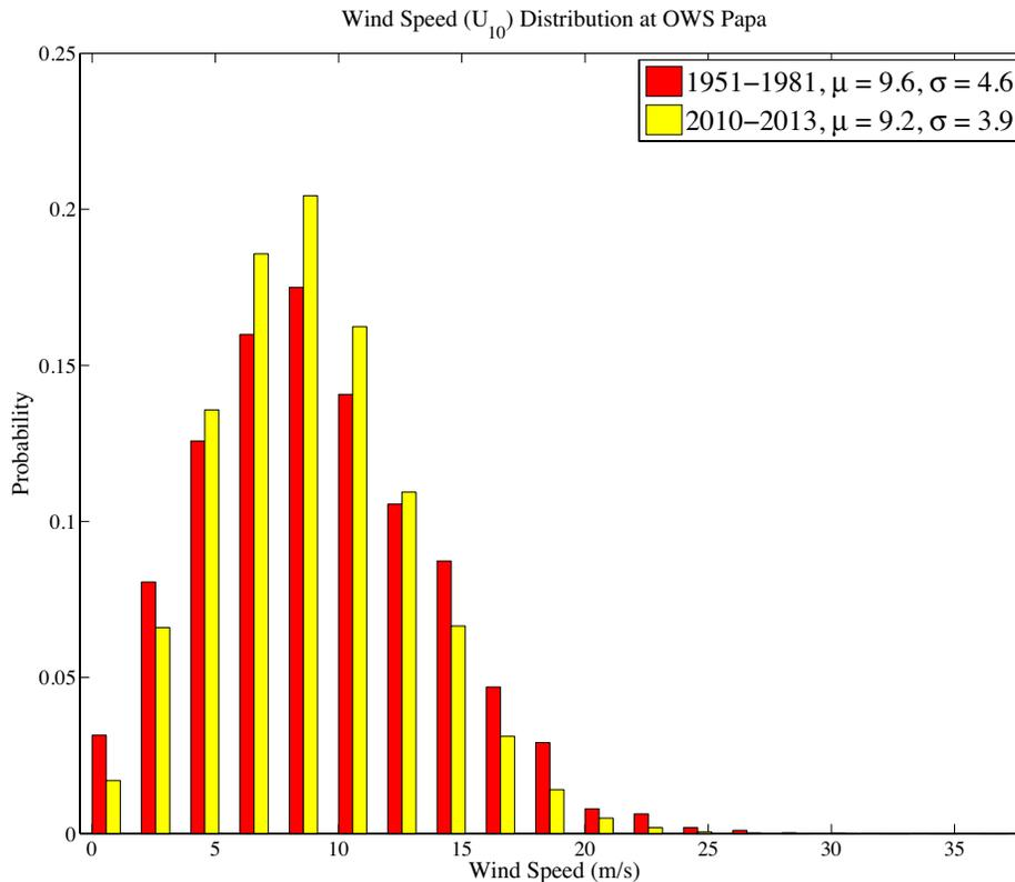
**Figure 2.** Statistical distribution of  $U_{10}$  speed at OSP. The statistical mean ( $\mu$ ) and standard deviation ( $\sigma$ ) show close agreement between the historical data (red) and the modern data (yellow).
