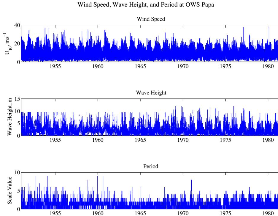
**Figure 1.** Full time series of wind speed, wave height, and wave period at OSP. *Note:* Period was reported using the following scale values: 0 (<5 s), 1 (6–7 s), 2 (8–9 s), 3 (10–11 s), 4 (12–13 s), 5 (14–15 s), 6 (16–17 s), 7 (18–19 s), 8 (20–21 s), 9 (>21 s).
