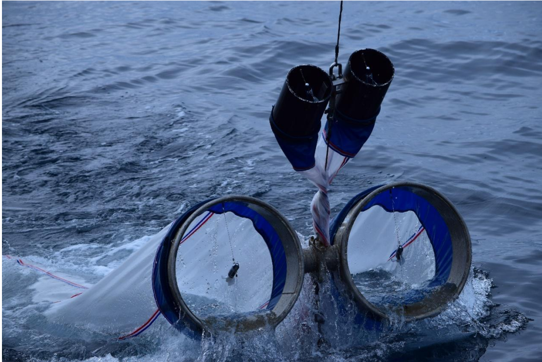
Retrieval of the bongo net used to sample the water column for zooplankton and larval fishes. Photo by Matthew Baker
