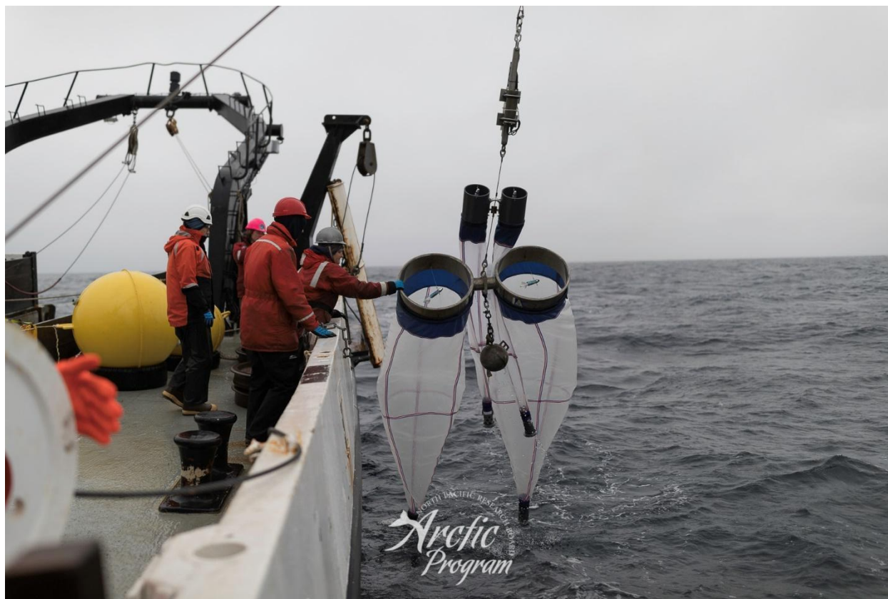
Libby, Sarah, Jordie, and Catherine recovering the Bongo net. Photo by Brendan Smith.
