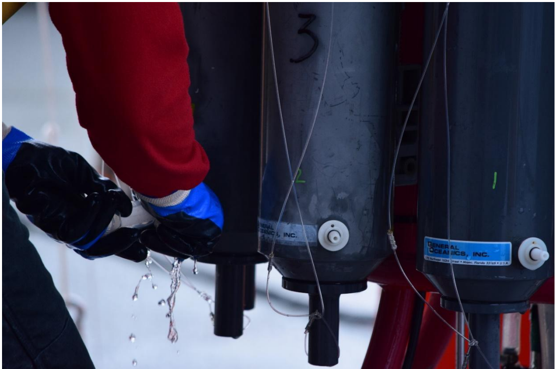
Water sample collection from Niskin bottles on the CTD rosette. Photo by Matthew Baker.
