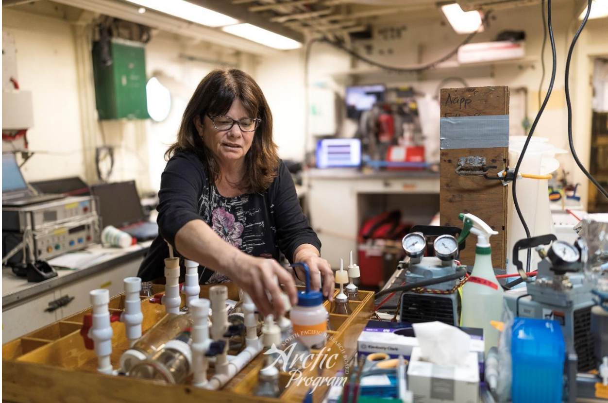
Lisa Eisner preparing to filter water from the CTD for chlorophyll. Photo by Brendan Smith.
