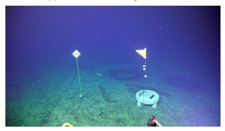
New benchmark AX-404 deployed at the top of the western caldera wall, during ROV Jason dive J2-1432.
