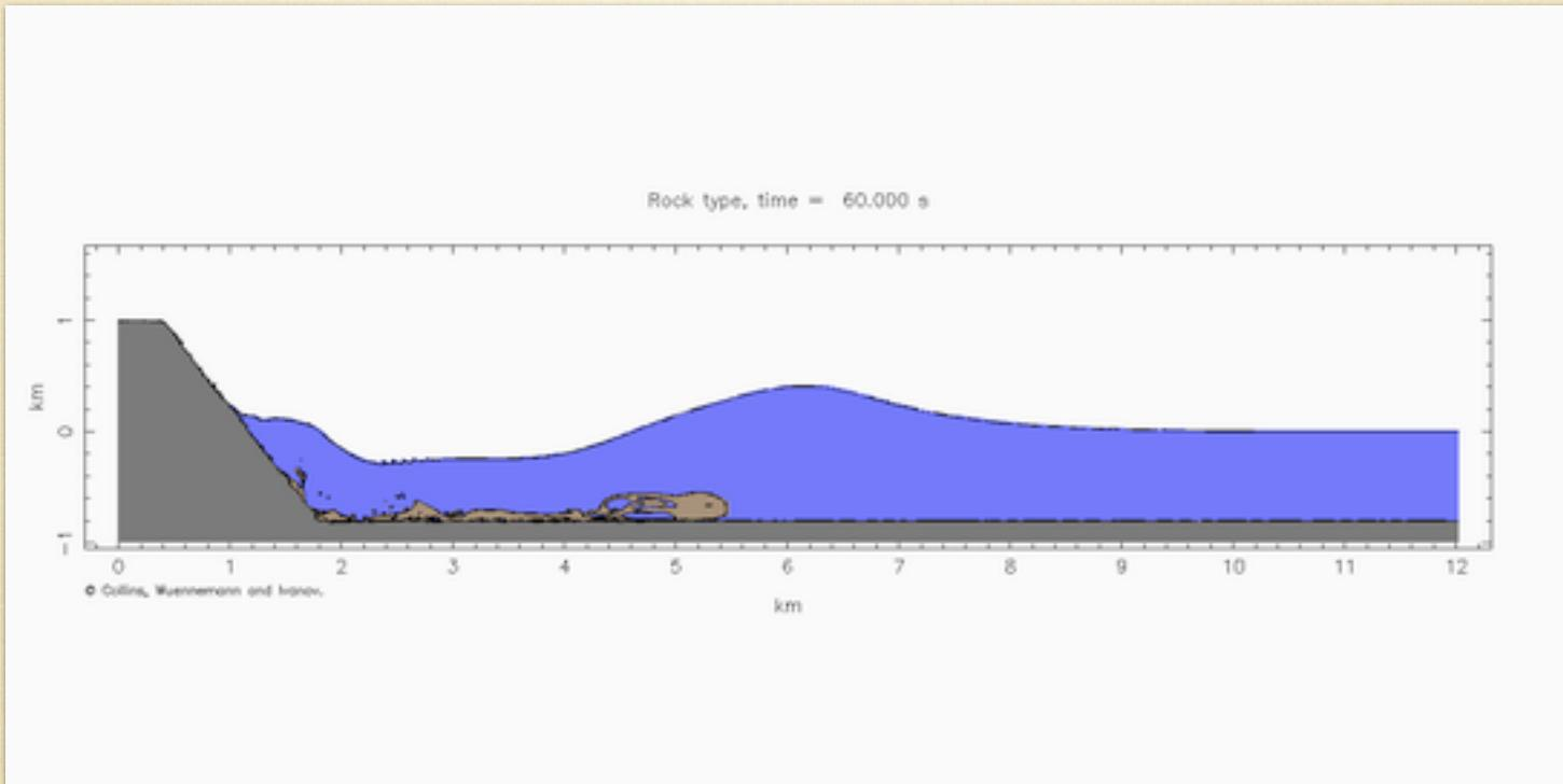
Large-scale landslide-generated tsunami model
