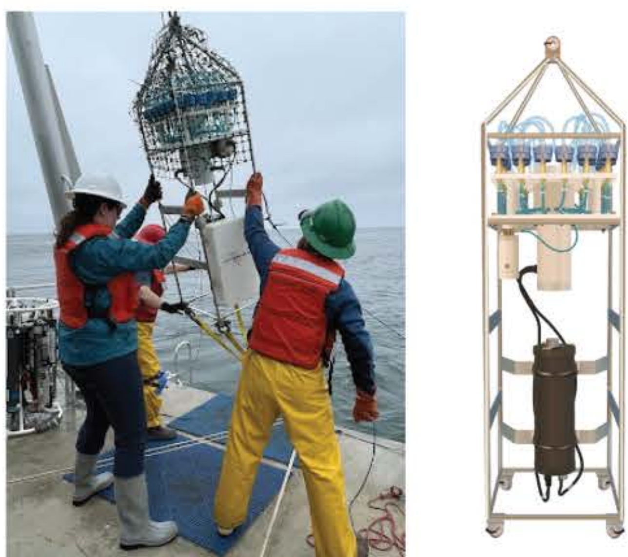
Automated eDNA sampler (PPS) Long-term moored deployments
